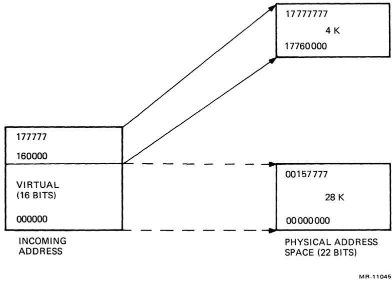
Figure 1-7 16-Bit Mapping
