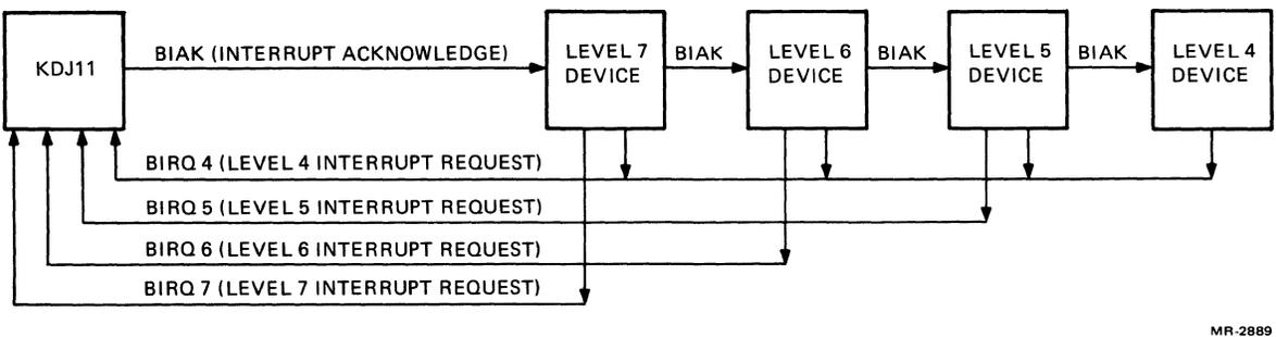
Figure 5-14 Position-Dependent Configuration
