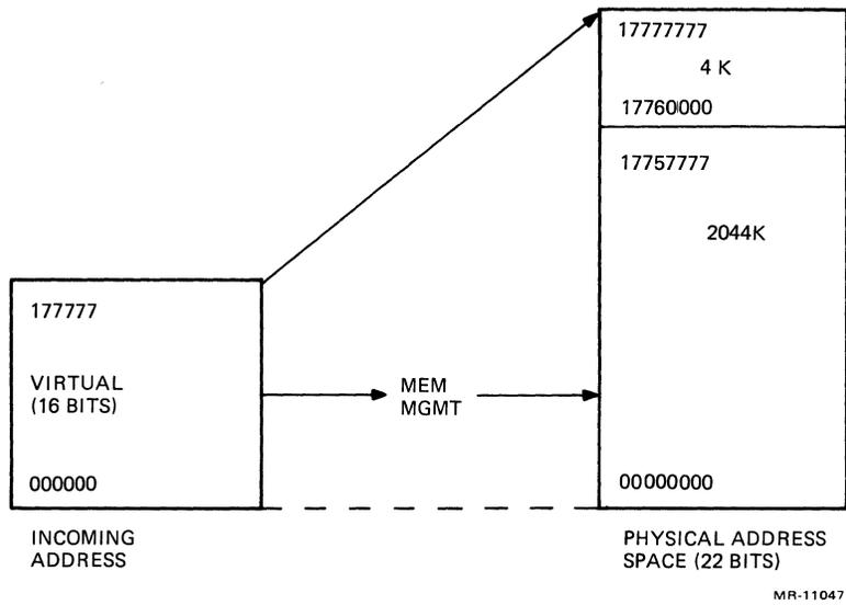
Figure 1-9 22-Bit Mapping
