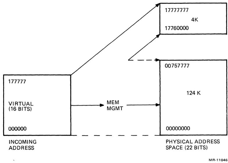
Figure 1-8 18-Bit Mapping
