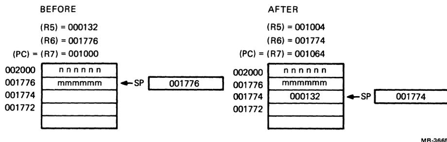
Figure 8-4 JSR Stack Condition Example
