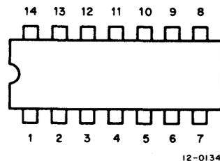
Figure 2-2 Integrated Circuit Pin Location - Top View
