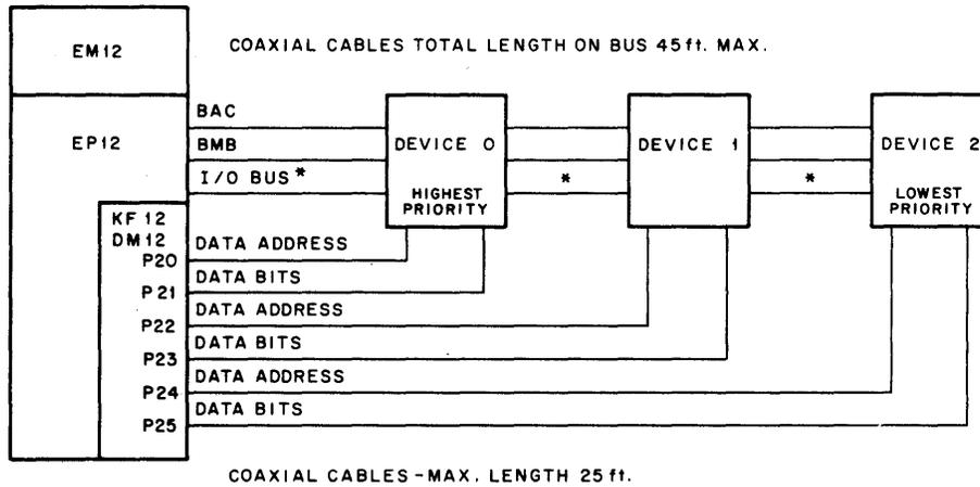
\* If the priority interrupt system is used in the KF12B this cable is connected separately from each device. (ref. BS-KF12-CAB).
