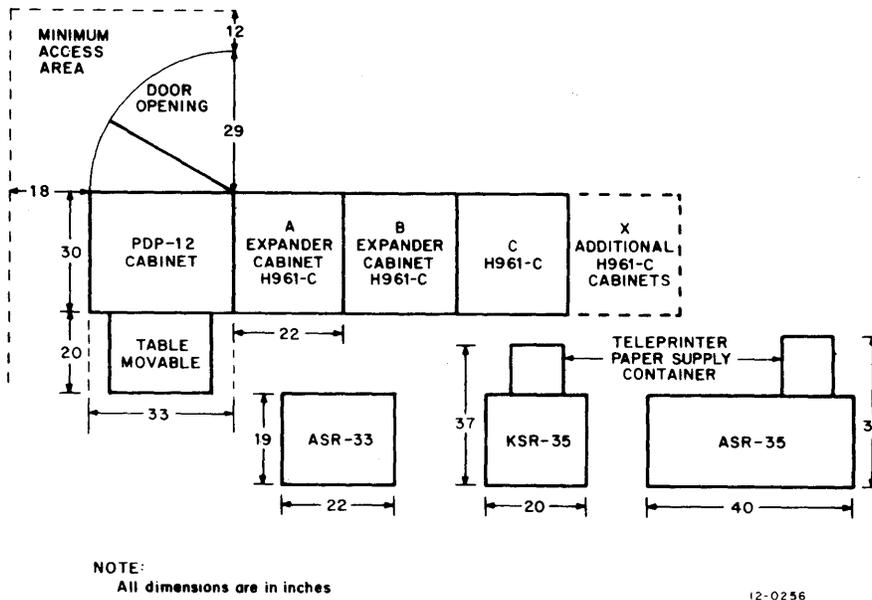
Figure 1-4 Minimum PDP-12 Equipment Floor Plan Requirements
