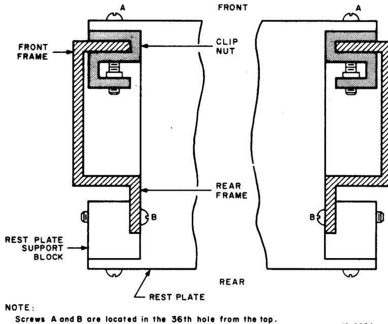
Figure 4-8 Top View of TU56 Rest Plate Assembly
