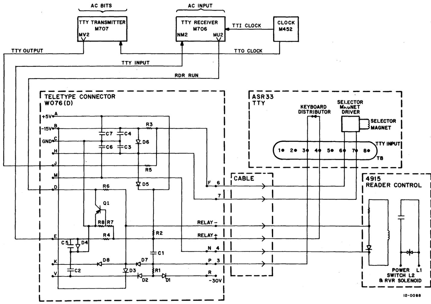
Figure 5-1 Teletype Connections
