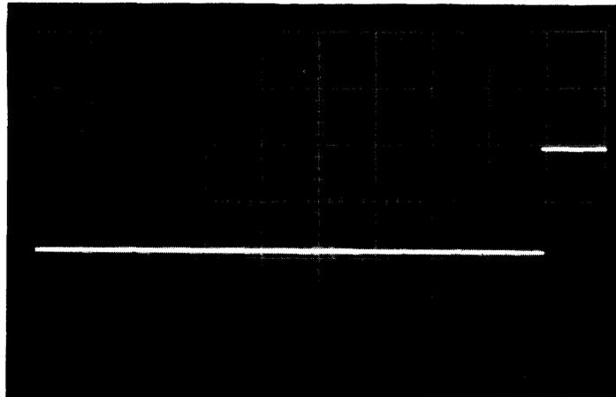
Figure 3-5 Teletype Clock (Sweep at .5 ms)
