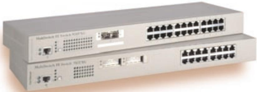
The MultiSwitch 924TXG and MultiSwitch 916TXG bring high-density switched Fast Ethernet with Gigabit Ethernet uplinks to the MultiSwitch 900 platform. Using the 12 Fast Ethernet channels across the MultiSwitch 900 backplane, the MultiSwitch 924TXG and MultiSwitch 916TXG enable MultiSwitch 900 users to allocate bandwidth among existing Ethernet and Fast Ethernet repeaters and
