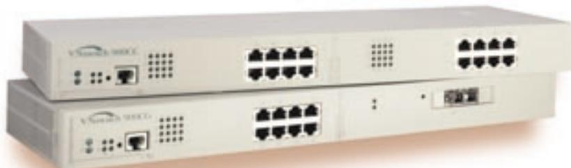
The VNswitch 900 product family of multi-layer, multi-technology enterprise-class switches is designed to provide layer 2 switching and layer 3 IP routing to the wiring closet. When combined with the MultiSwitch 900 chassis, multiple VNswitch 900s can be connected together by one of three 400mbs
