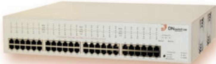
A manageable, stand-alone 48-Port switch, the DNswitch 248 connects workstations and other network devices on networks of all sizes.
