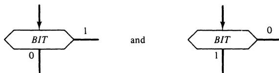
we could compare the current value of the toggle switch with a reference value supplied by the architecture and not by the ASM chart itself. If we call this reference value for a particular bit *REF*, then the ASM chart would contain
