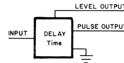
Delay. A monostable multivibrator which produces one or two level outputs while it is timing out, and then may trigger a Pulse Amplifier. Operating time adjustable.
