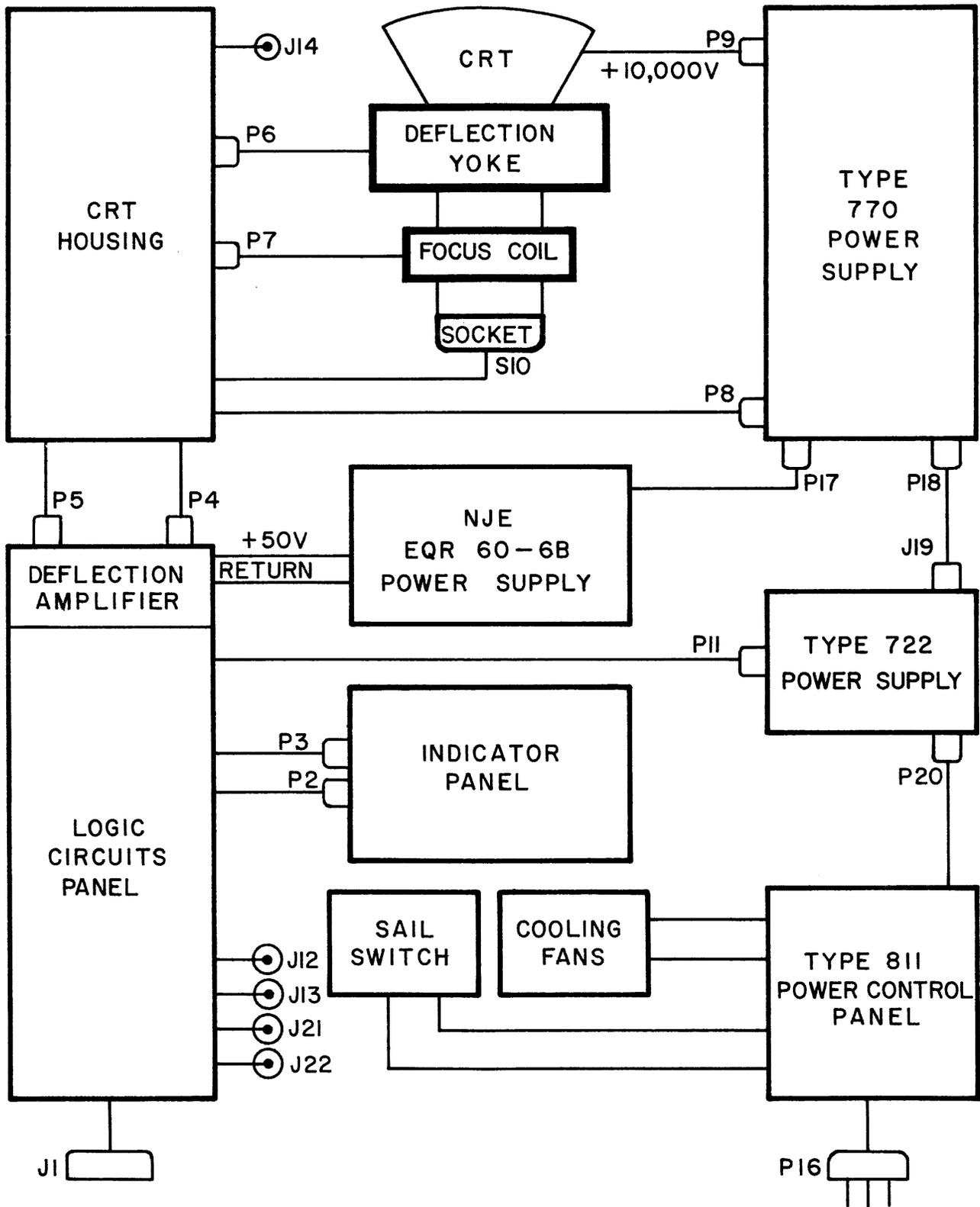
FIGURE 5-6 TYPE 30E CABLE AND WIRING DIAGRAM
