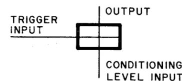
Capacitor-Diode Gate. Differentiates the input if the conditioning level has had the proper voltage for approximately three microseconds.
