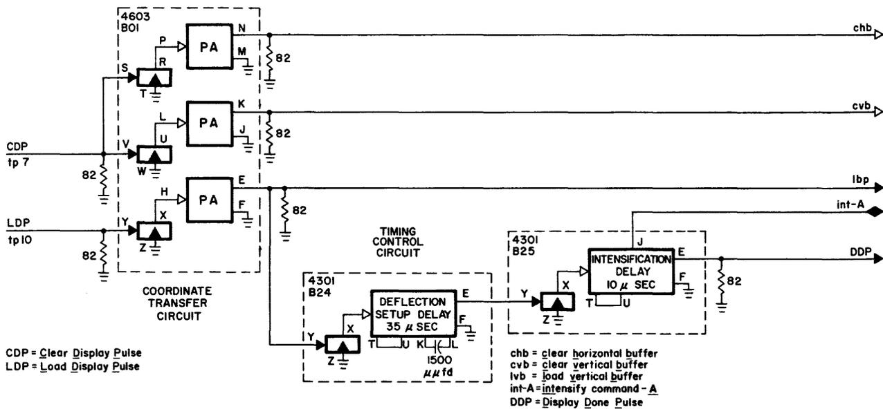
Figure 3-5 Control and Timing Circuit Logic Block Diagram
