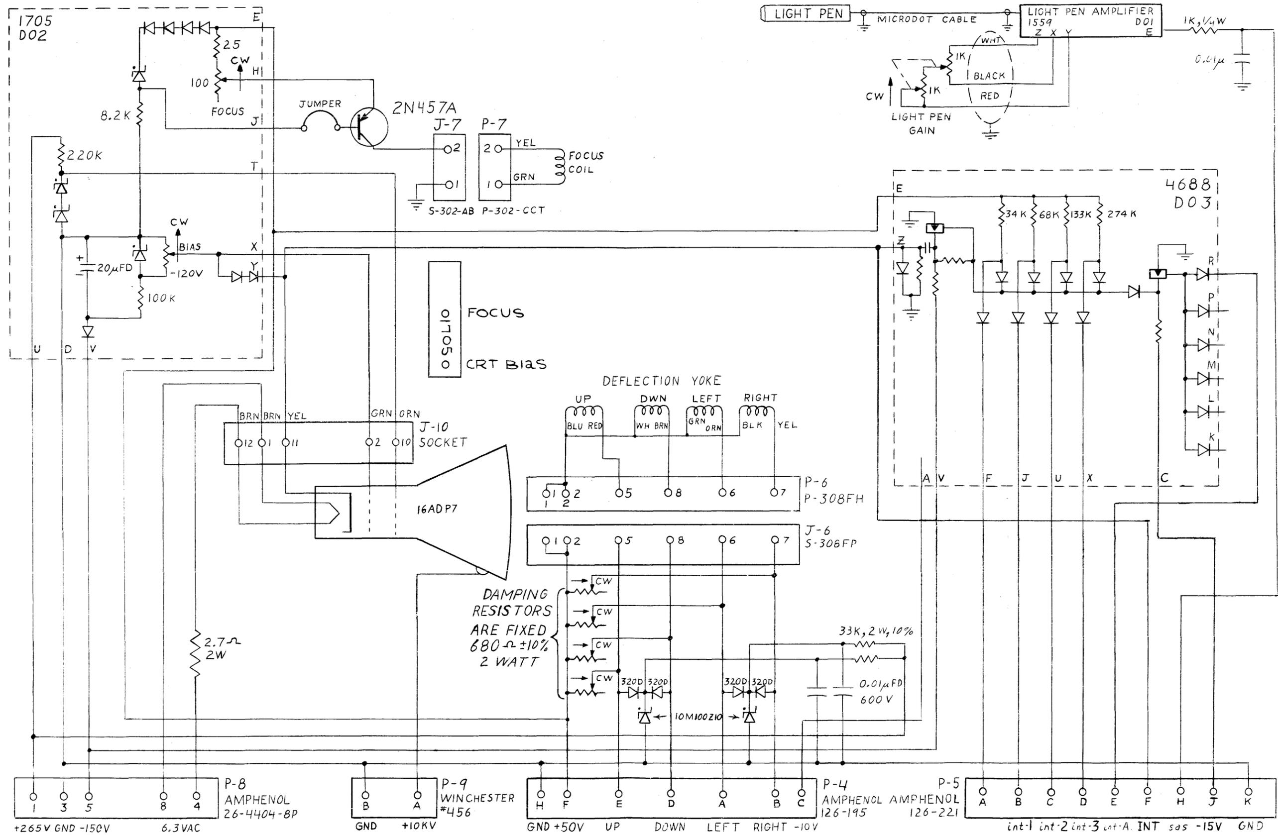
Figure 5-3 Type 30 Display Housing Schematic
