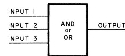
Logic Gate. May be either AND or inclusive OR, depending on polarity of inputs and output. Number of inputs unlimited.
