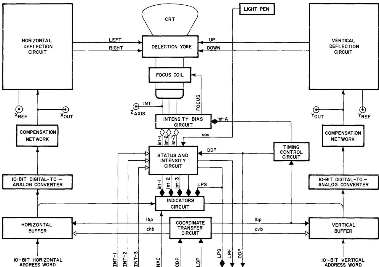
Figure 3-1 Type 30E Block Diagram
