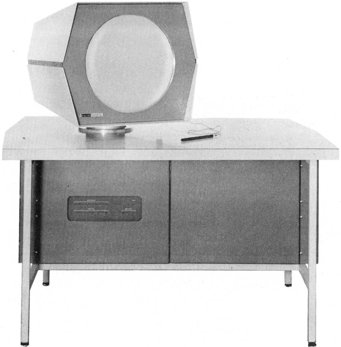
Figure 1-1 Type 30 Precision CRT Display
