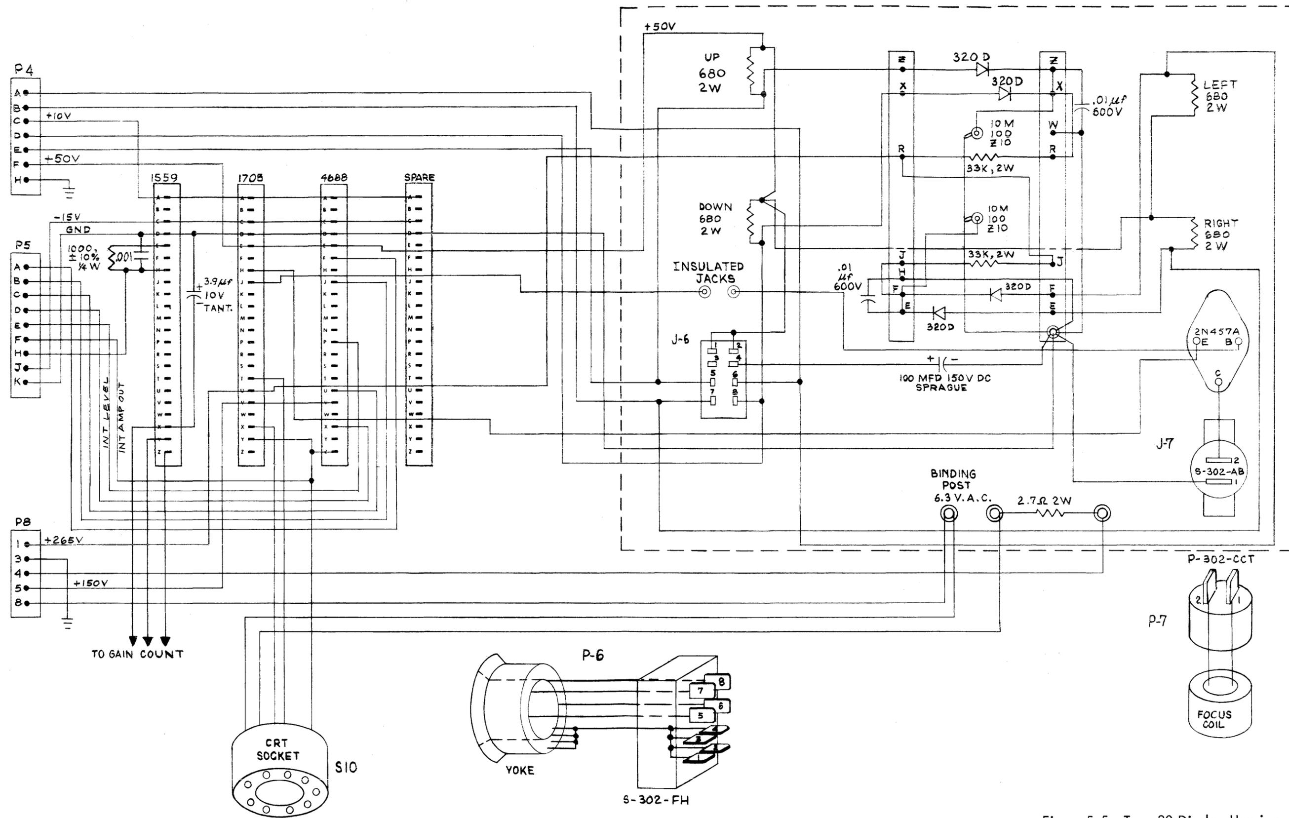
Figure 5-5 Type 30 Display Housing
