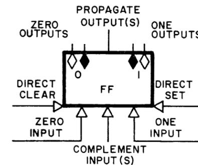
Flip-Flop. A bistable multivibrator with numerous inputs and two outputs, which may be buffered. Outputs shown twice, with diamonds indicating voltage levels in each state. Positive pulses from ground to +2.5 volts required to set or clear on inputs. A complement input changes the state regardless of the previous state, and may generate a propagate pulse output.
