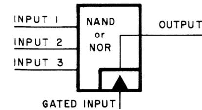
NAND or NOR Logic Gate. Same as an AND or OR Logic Gate with an inverter which may be gated. Output polarity opposite to input polarities.
