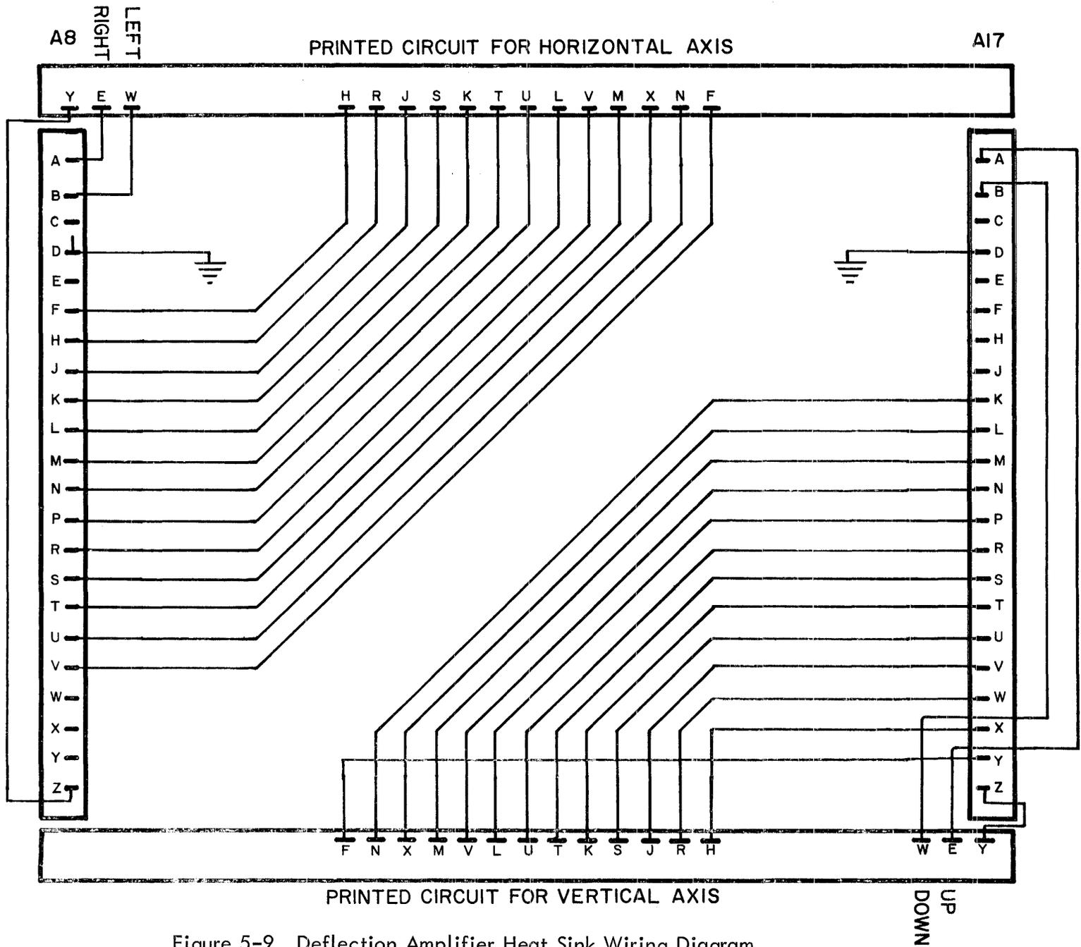
Figure 5-9 Deflection Amplifier Heat Sink Wiring Diagram
