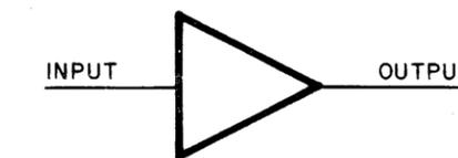
Analog Amplifier. Any amplifier that operates over a continuous voltage range. May have single or multiple inputs and/or outputs. Generally requires different voltages.
