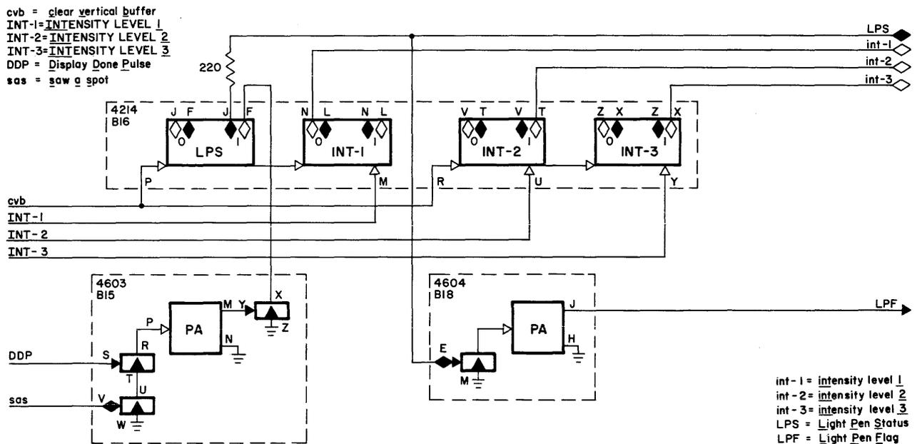
Figure 3-6 Status and Intensity Circuit Logic Block Diagram
