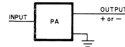
Pulse Amplifier. Amplifies and standardizes DEC pulses. Output is from a pulse transformer, giving either positive or negative pulses depending on which side is grounded.
