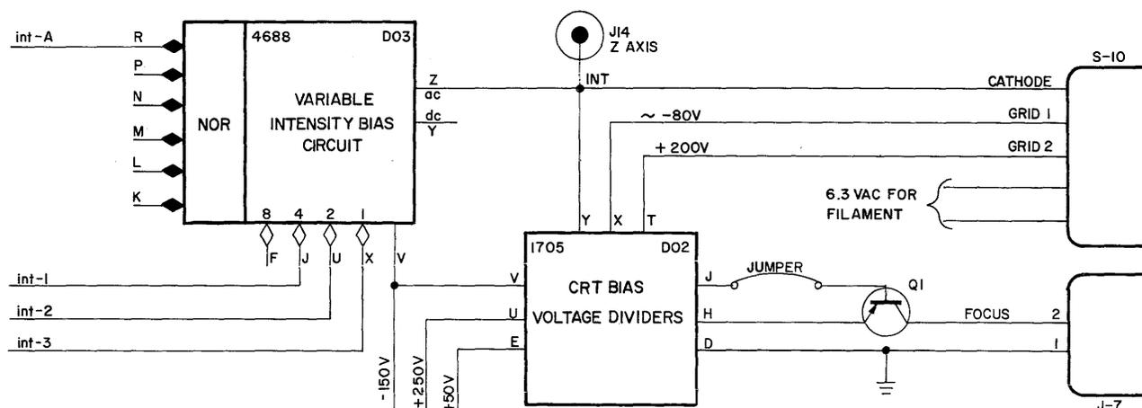
Figure 3-7 Intensity Bias Circuit Logic Block Diagram
