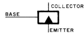
Inverter. A transistor in common-emitter configuration, with biased input on its base. Emitter must be at ground to conduct. Ground input cuts it off and -3 volt input saturates it. Delay = 20 nanoseconds.
