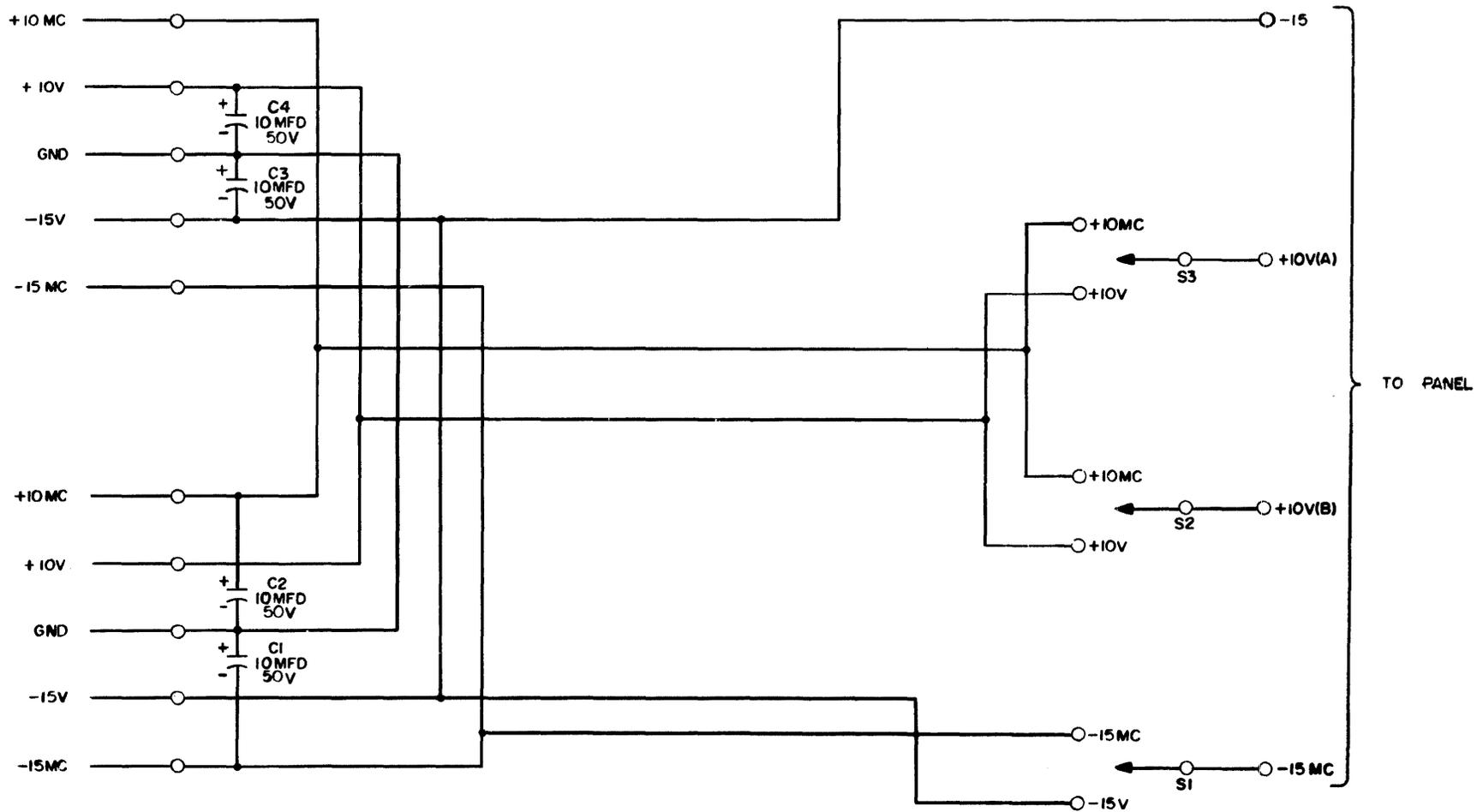
Figure 5-8 Logic Circuits Power End Panel Schematic
