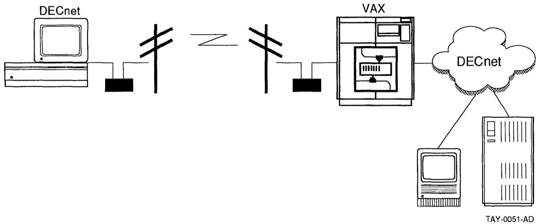
Figure 1-3 shows a typical asynchronous configuration. This configuration uses a telephone line between a Macintosh computer that runs DECnet software and a VAX computer that is a DECnet router. 2400 baud modems and RS-232C cables connect the computers to the telephone line.
