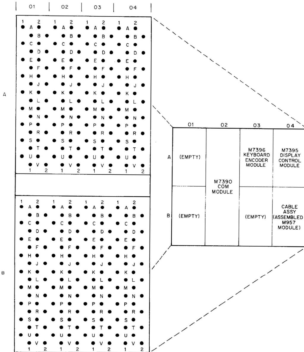
Figure 5-5 RT02-A Module Connector Block (Wiring Side)
