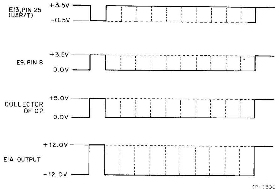
Figure 5-7 M7390 Module Serial Output Example Format
