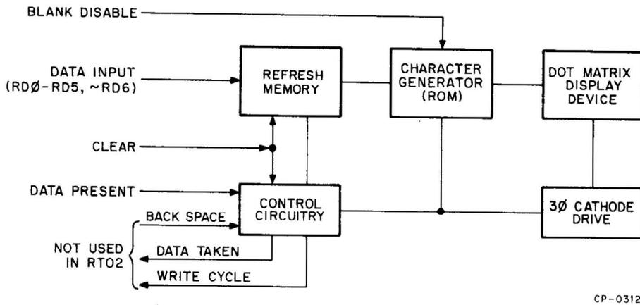
Figure 4-10 Display Panel, Block Diagram
