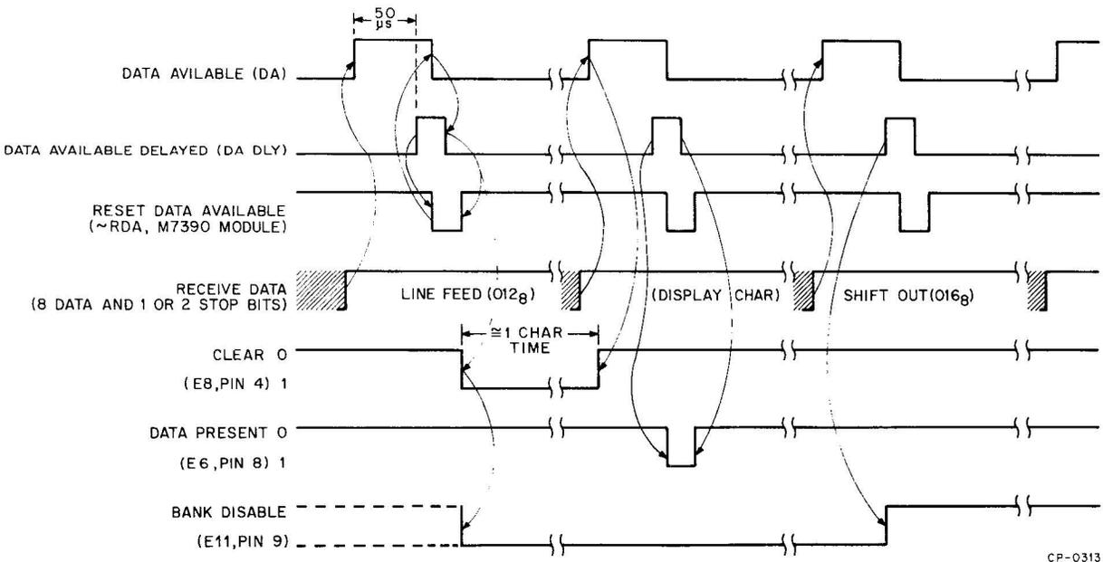
Figure 4-9 Control Signal Timing, M7395 Display Control Module
