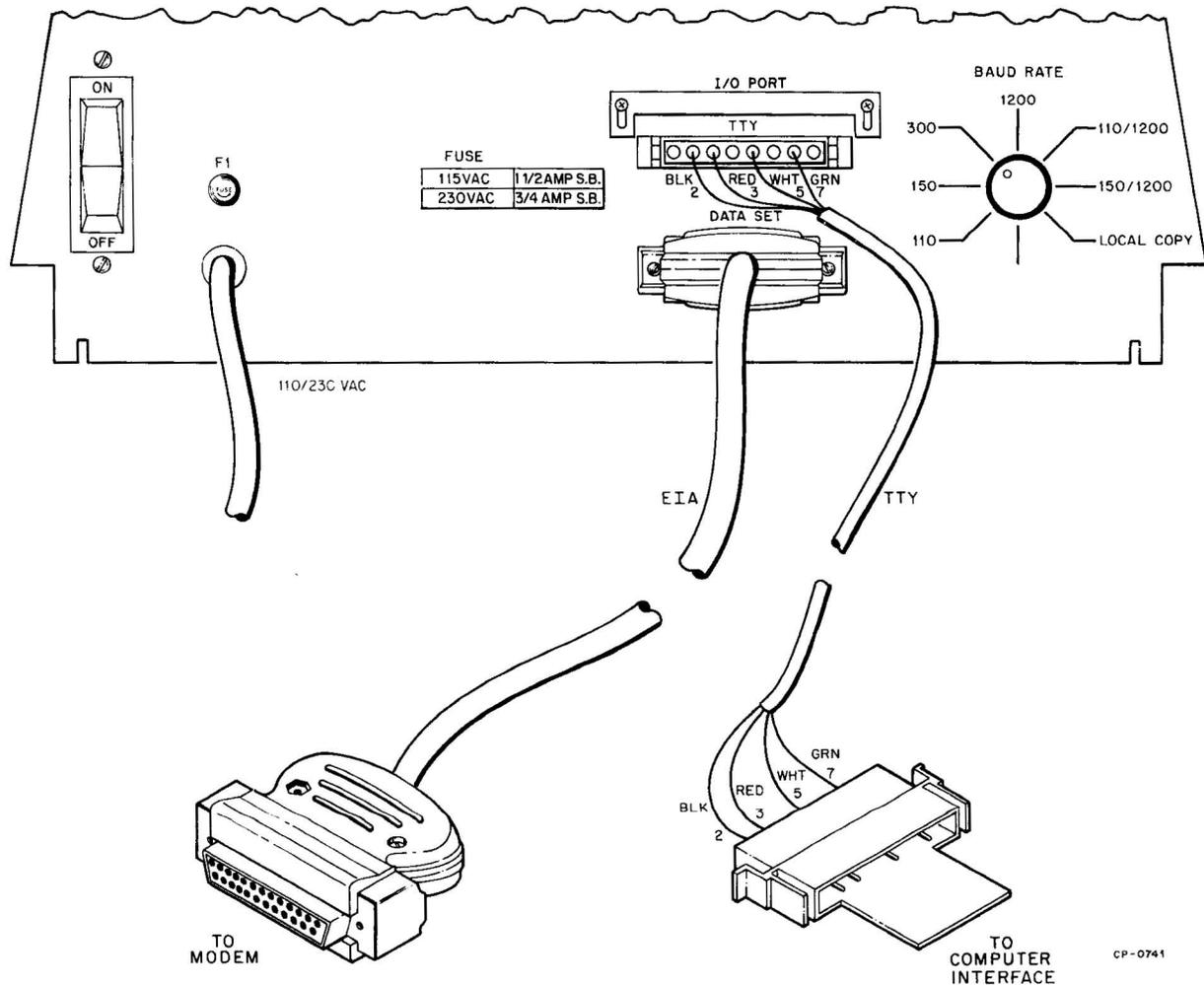
Figure 2-2 RT02-A Rear Panel and Connector Cables
