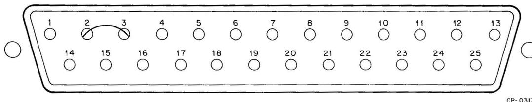
Figure 2-6 EIA Connector Pin Assignments
