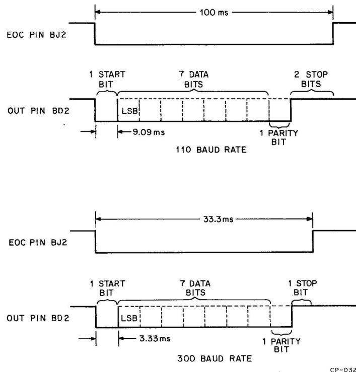
Figure 1-4 110 and 300 Baud Rate, Serial Output Examples (M7390 Communications Module)
