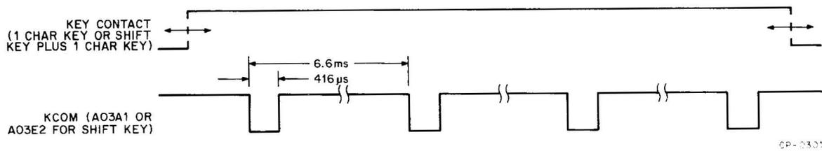
Figure 5-4 Keyboard Timing
