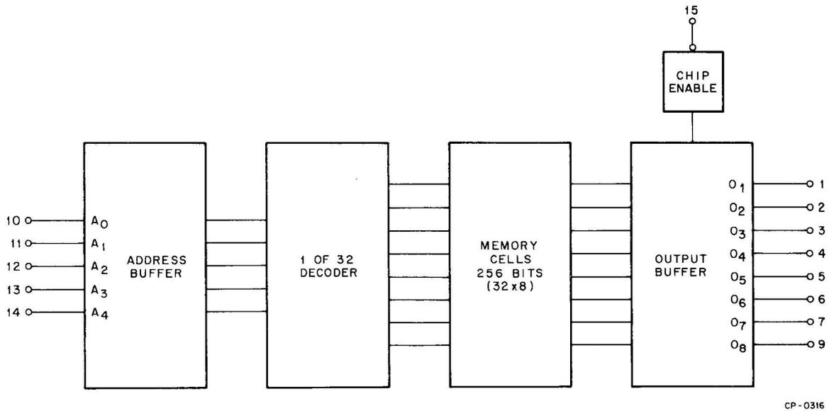
Figure 4-3 Programmable Read-Only Memory (PROM), Block Diagram
