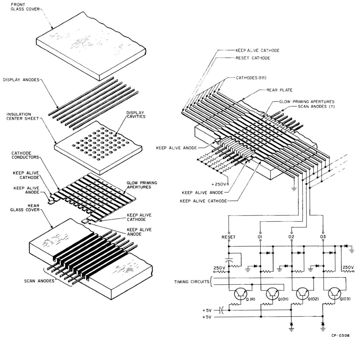
Figure 4-13 Construction of Self-Scan Panel Display
