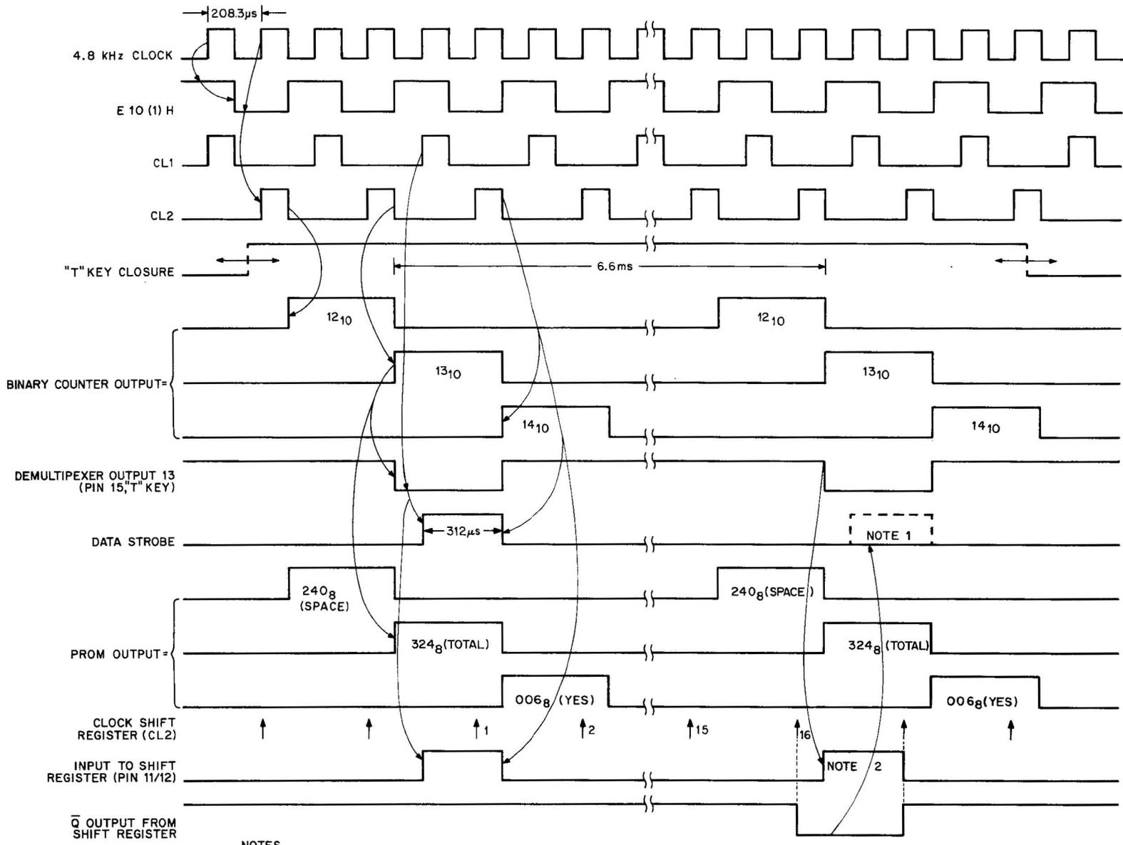
Figure 4-2 M7396 Keyboard Encoder Timing (Example: TOTAL Key)
