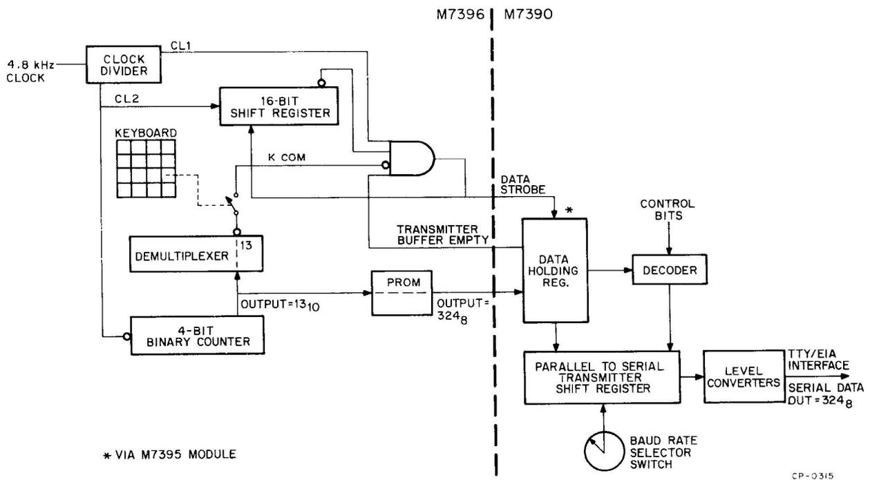
Figure 4-4 Transmit Mode Block Diagram (Example: TOTAL Key)
