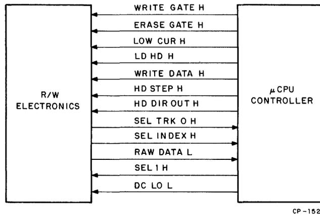
Figure 5-5  $\mu$ CPU Controller to Read/Write Electronics Signals
