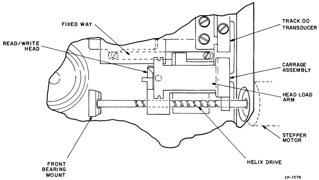
Figure 5-26 Positioning Mechanism
