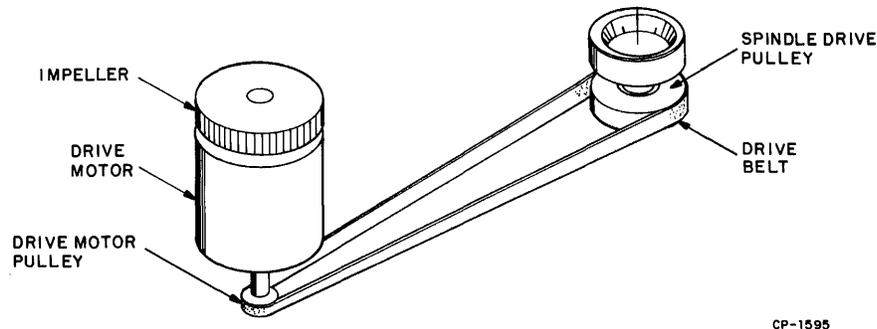
Figure 5-24 Drive Mechanism
