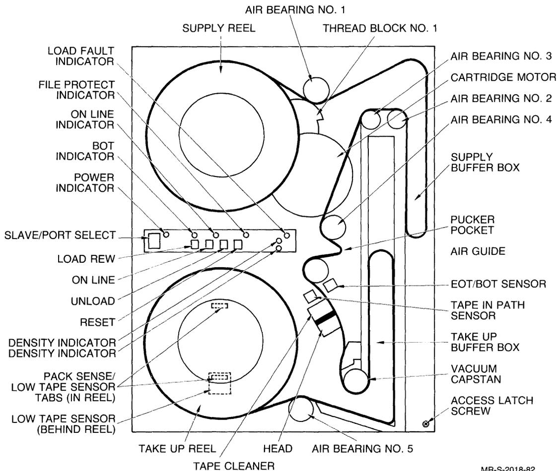
**Figure 4-7: TU77, TU78, or TU79 Tape Path and Controls**
