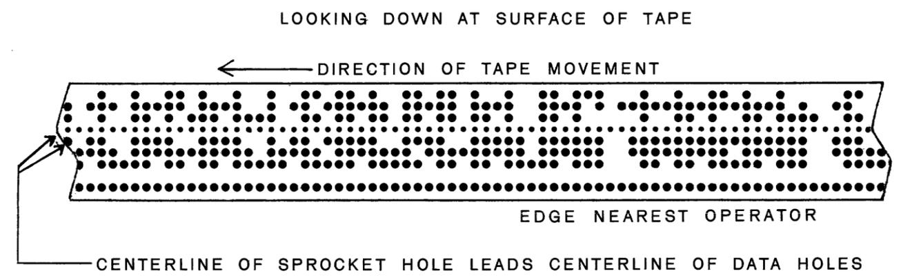
Figure 11-9 Correct Orientation for Loading Paper Tape
