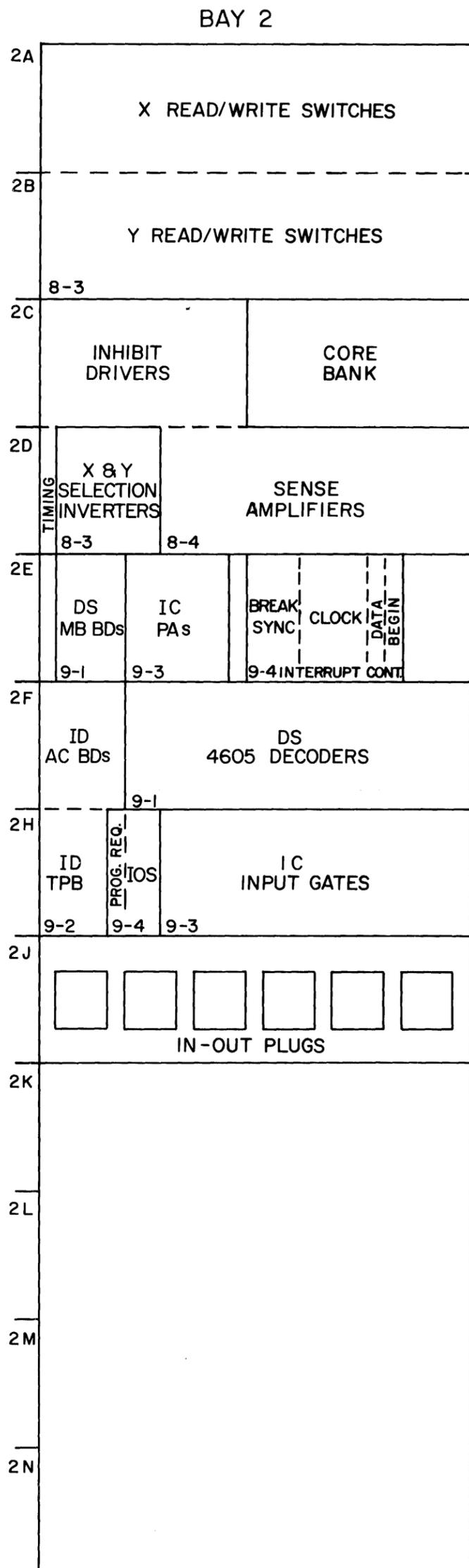
Figure 11-1 PDP-4 Detailed Logic Layout
