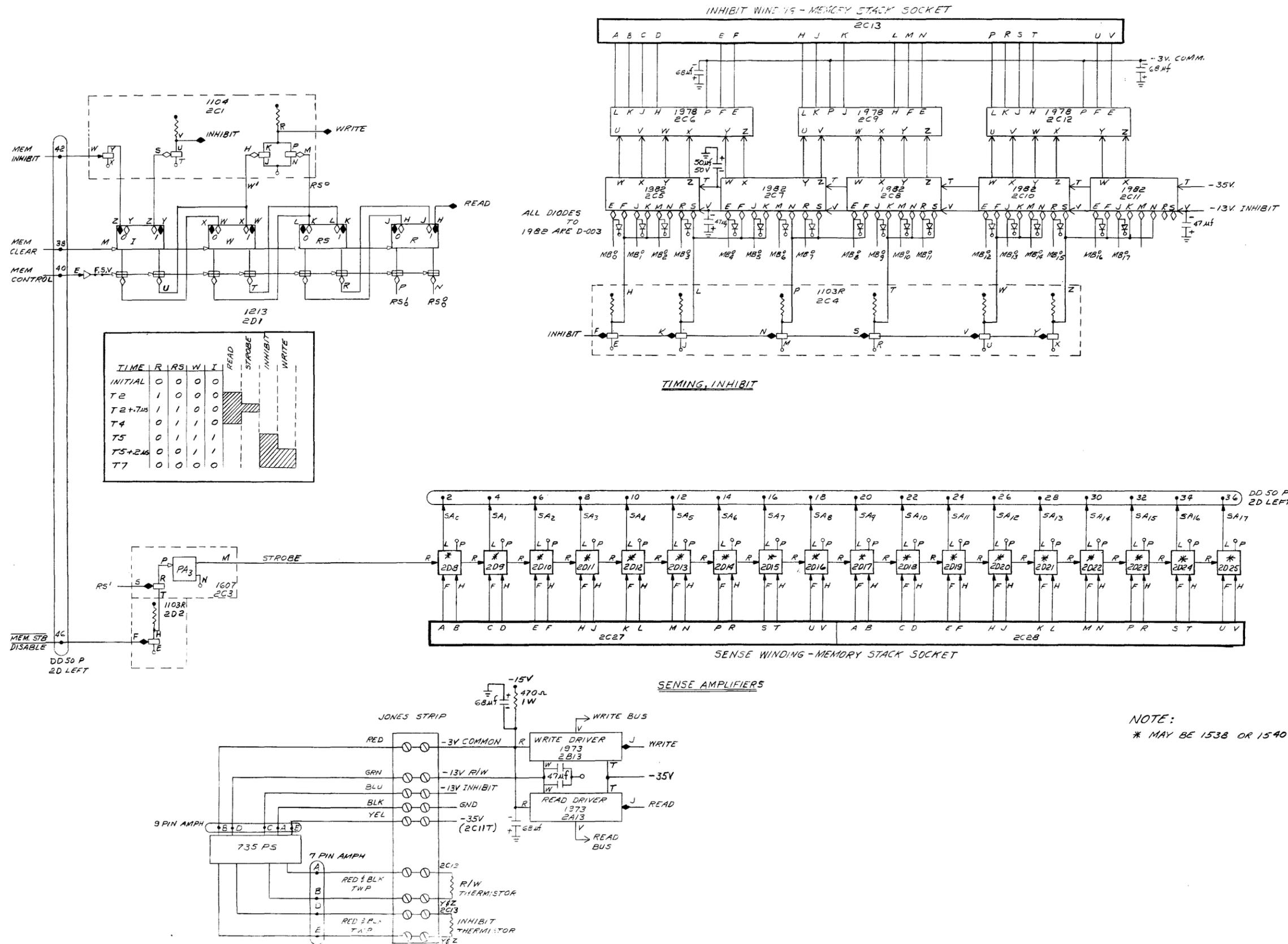
Figure 8-4 Memory: Timing, Inhibit Driving, Read Sensing
