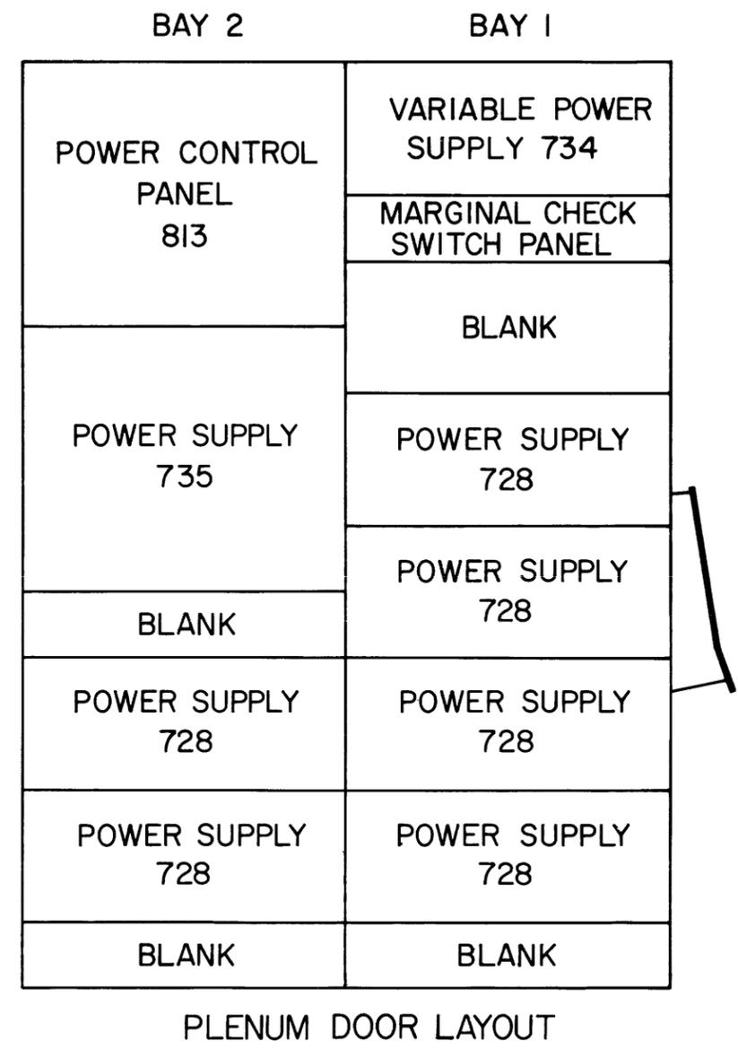
Figure 2-6 PDP-4 Layout Diagram
