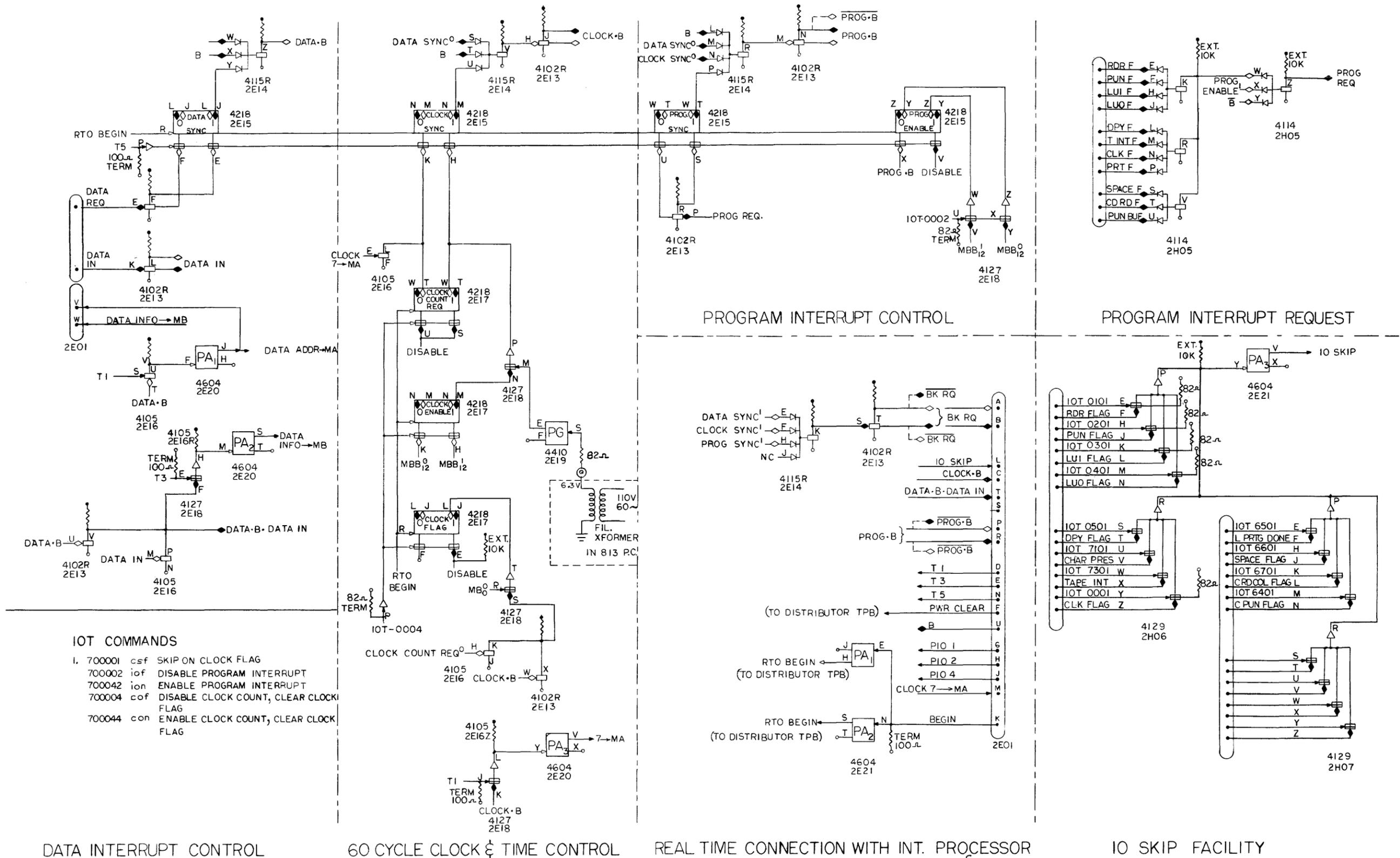
Figure 9-4 Data, Clock and Program Interrupt Logic, In-out Skip Logic
