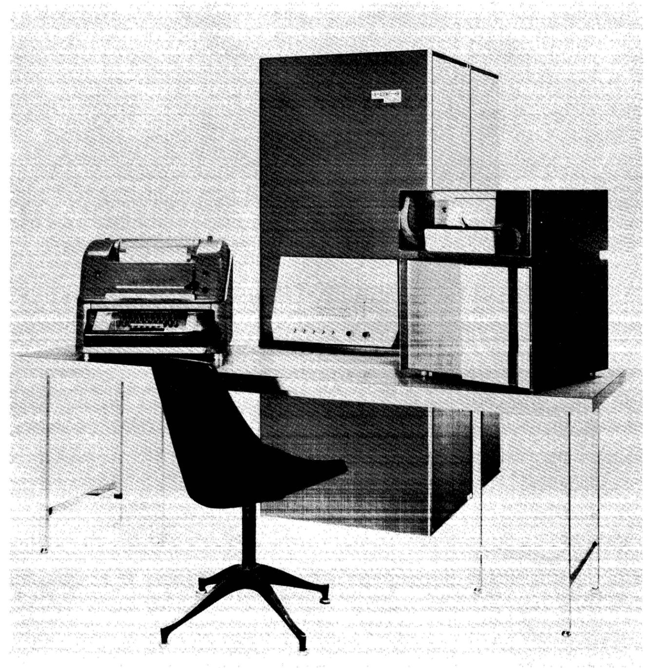
Figure 2-2 PDP-4 with Reader, Punch and Keyboard/Printer
