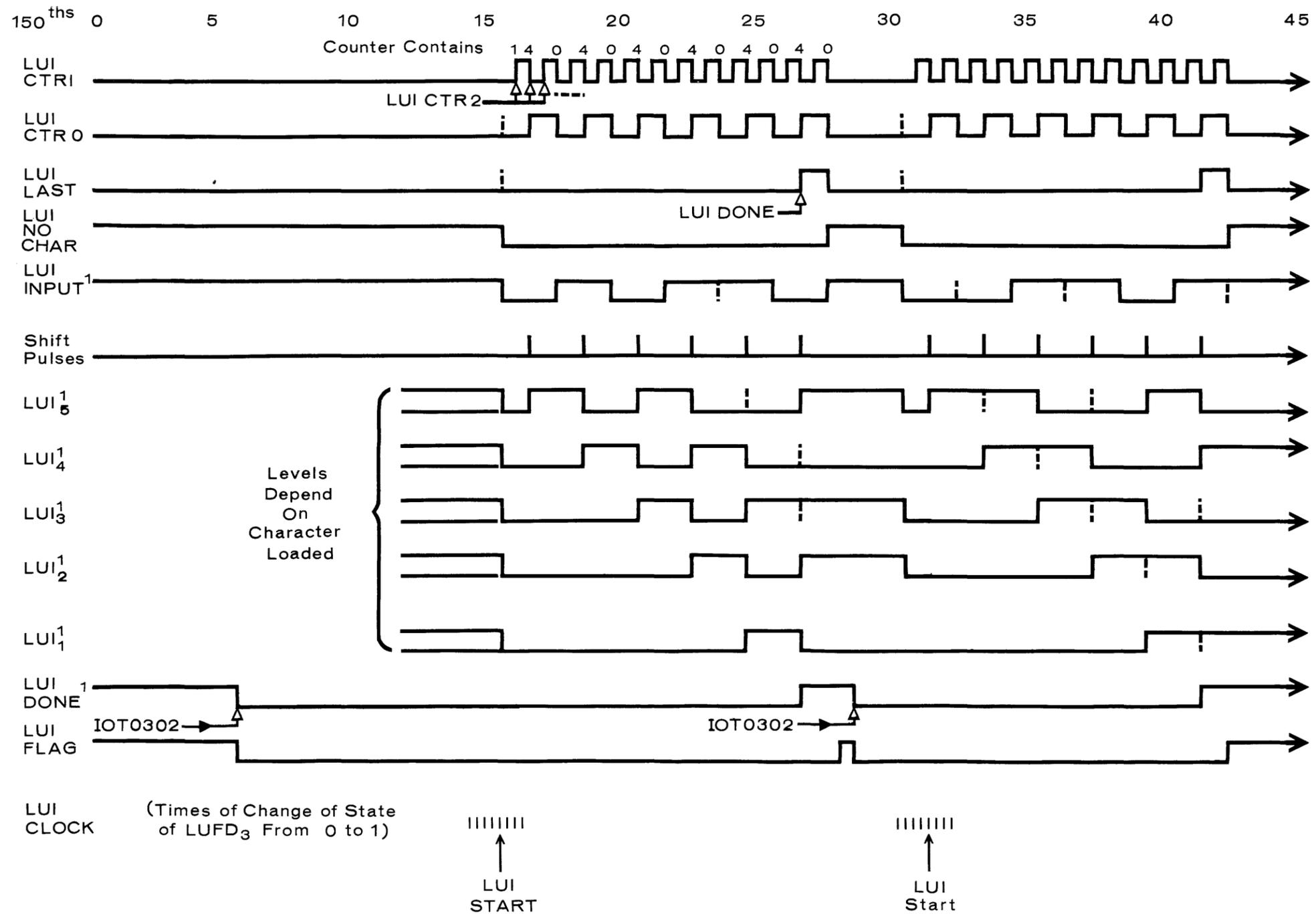
Figure 9-9 Timing Diagram: Incoming Line Unit
