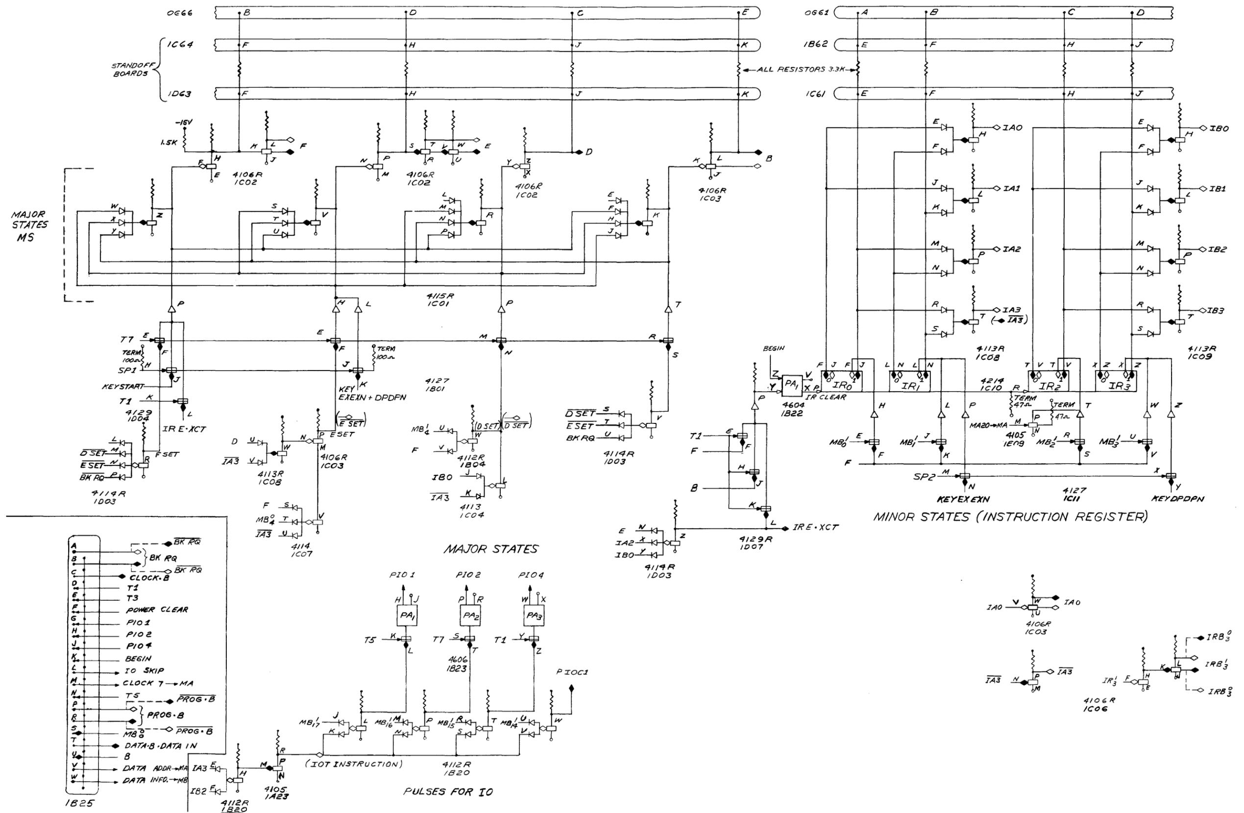
Figure 6-2 States, In-out Transfer Control
