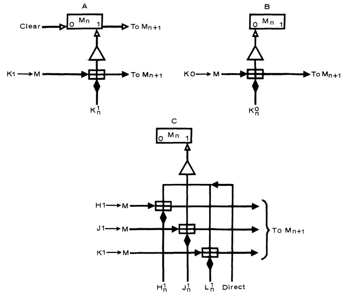
Figure 4-4 Transfer Logic
