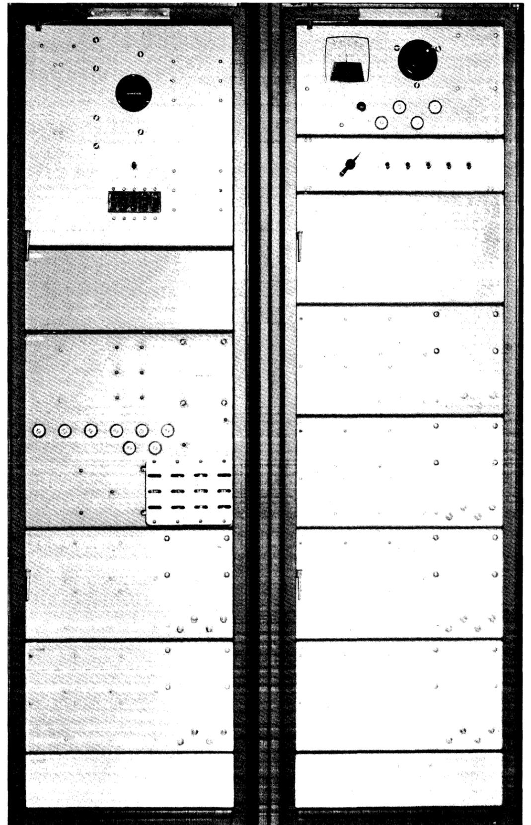
Figure 2-4 Plenum Doors, Back View of PDP-4 Bays
