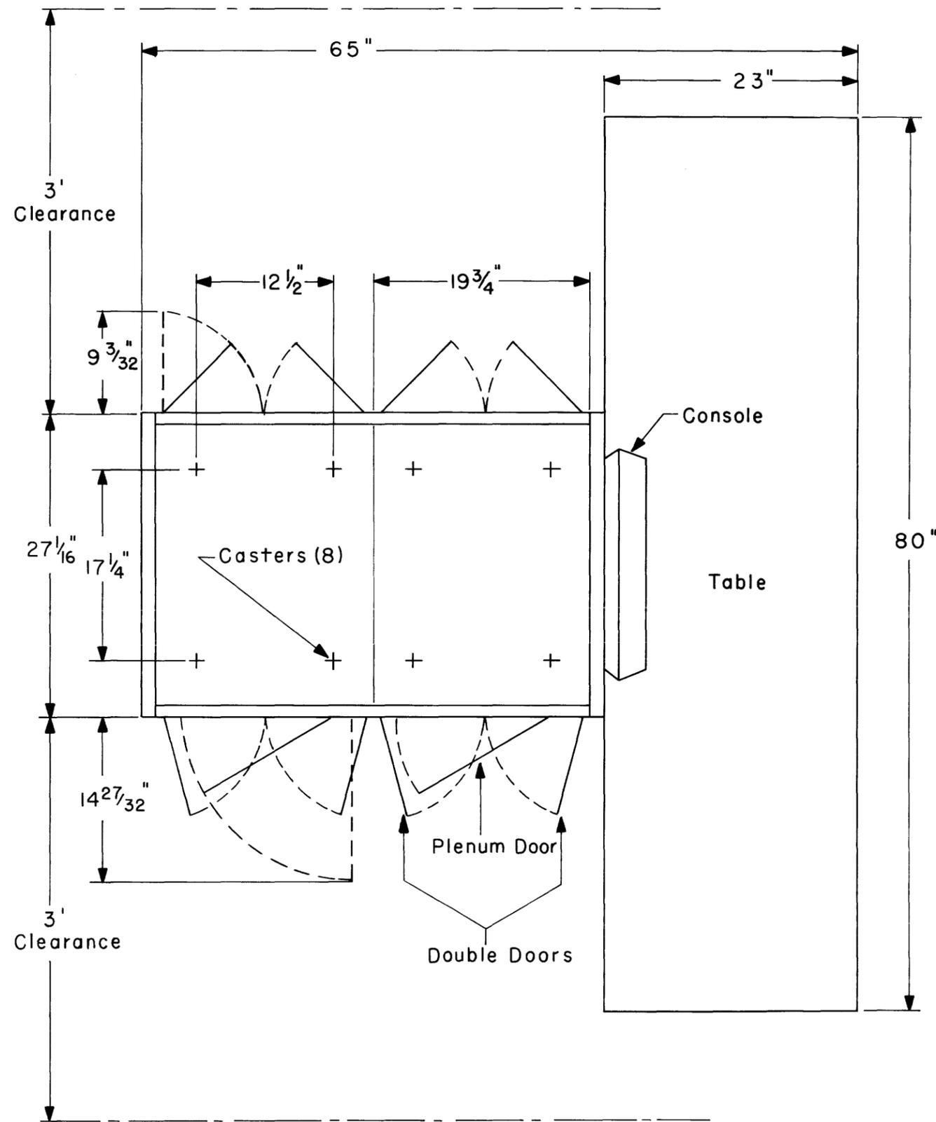
Figure 3-1 PDP-4 Top View
