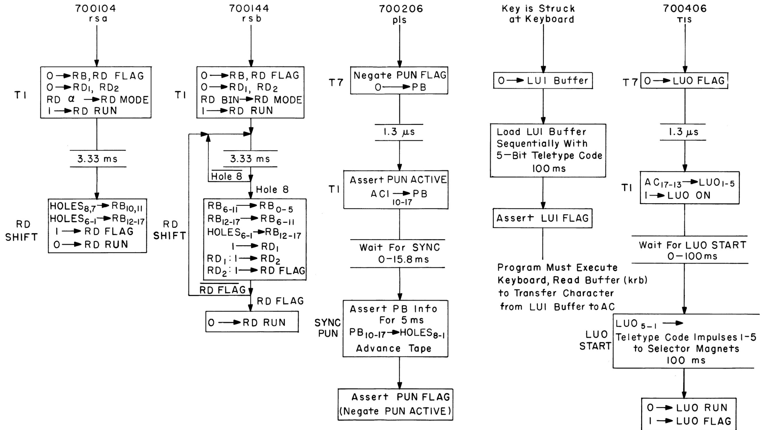
Figure 4-7 Flow Chart: Input-Output Operations
