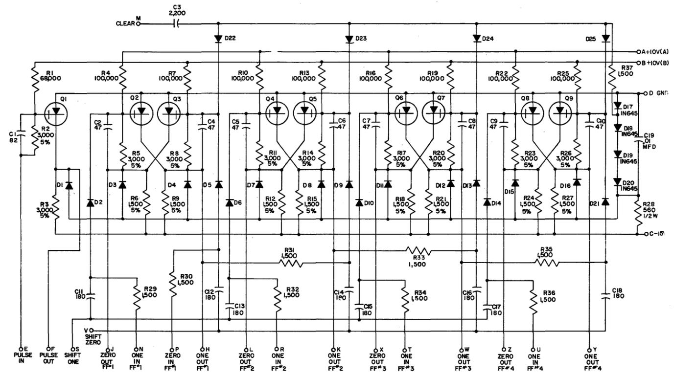
UNLESS OTHERWISE INDICATED: RESISTORS ARE 1/4W, 10%. CAPACITORS ARE MMFD. DIODES ARE 1N276. TRANSISTORS ARE 2N1427
