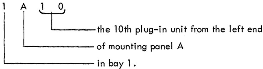
Terminal designations are formed by adding the pin letter to the plug-in unit location code described above.
