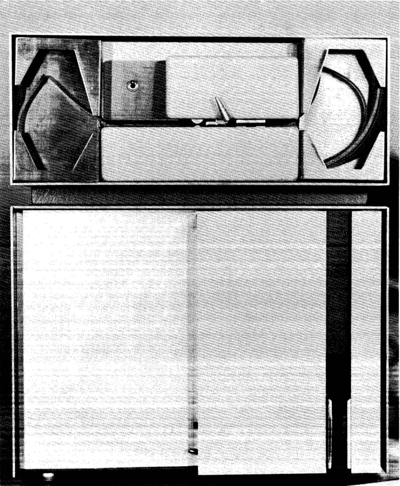
Figure 5-5 Paper Tape Reader (mounted on punch cabinet)
