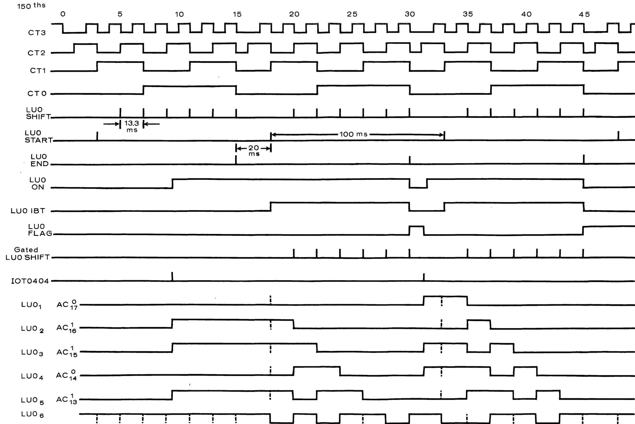
Figure 9-8 Timing Diagram: Outgoing Line Unit
