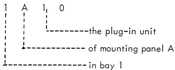
Terminal designations are formed by adding the pin letter to the plug-in unit location code described above.
