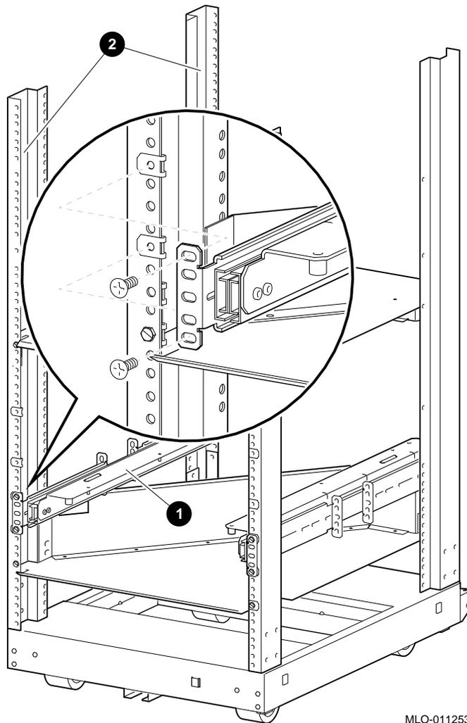
**Install the Chassis Slide Support Brackets**
