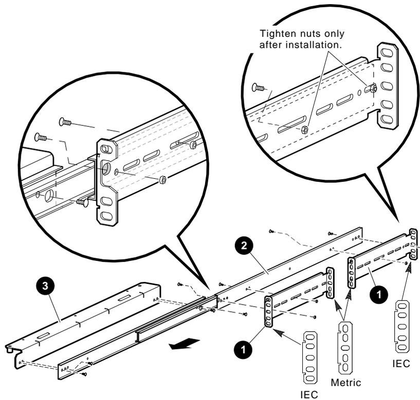
**Install the Right Side Chassis Slide Assembly**
