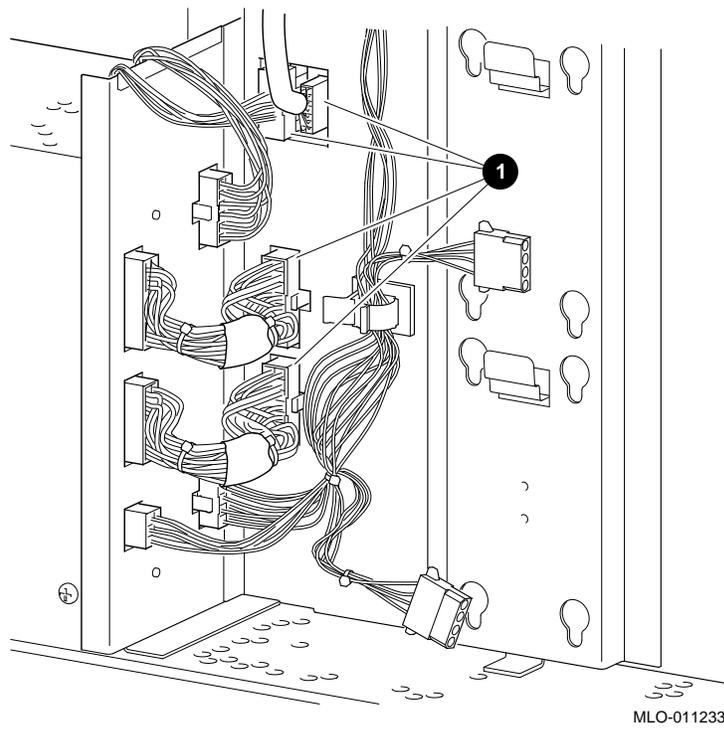
Figure 8-21 shows the TURBOchannel connections for the DEC 3000 Model 800/800S AXP system.
