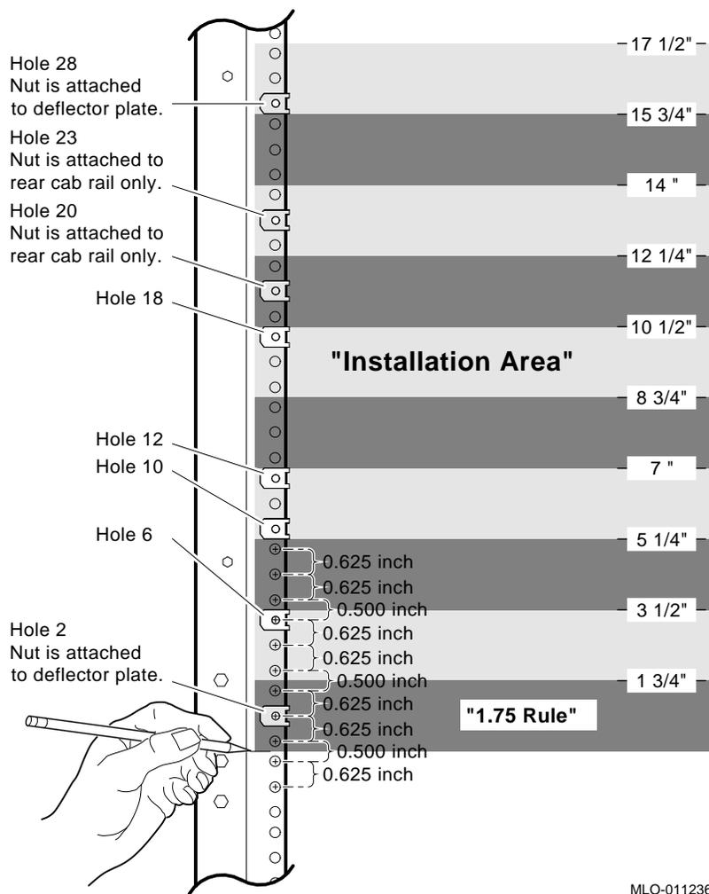
**Assemble the Top Air Deflector and Baffle Subassembly**
