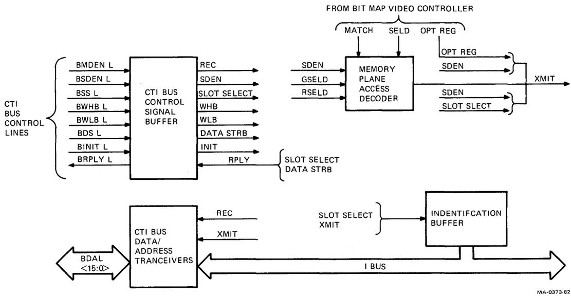
Figure 7-23 CTI BUS Interfaced Circuit Operation (Option Module)
