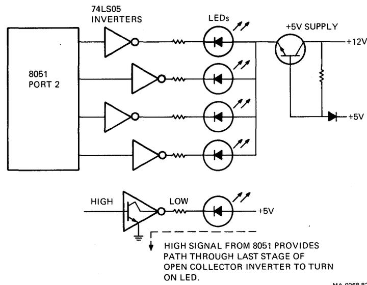
Figure 6-9 Indicator (LED) Control Circuit
