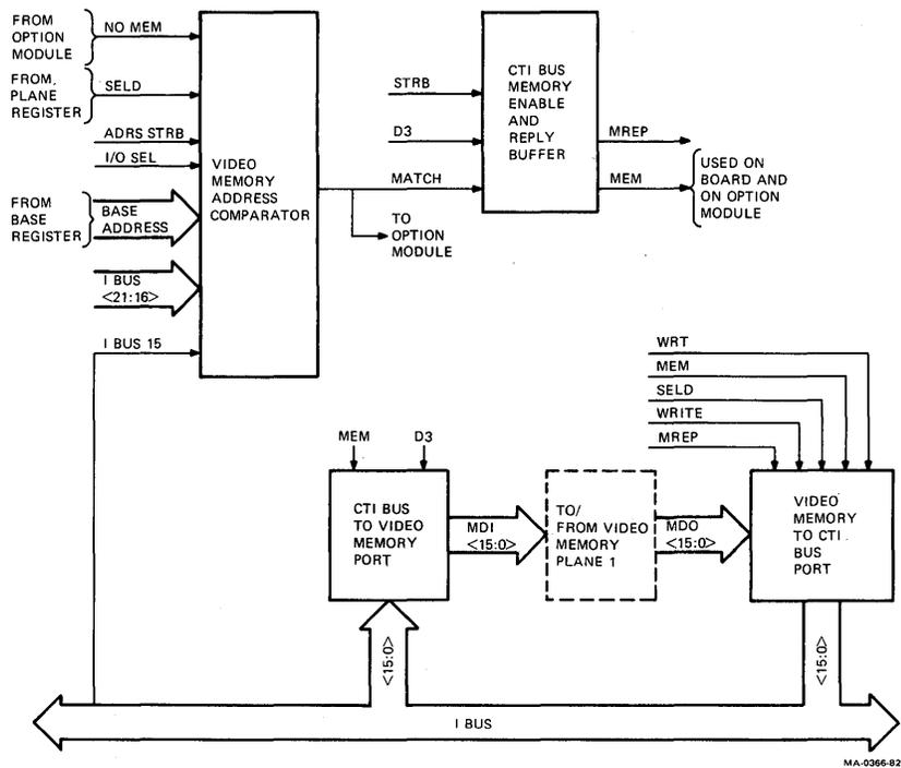
Figure 7-16 CTI BUS Video Memory Access Circuit Operation
