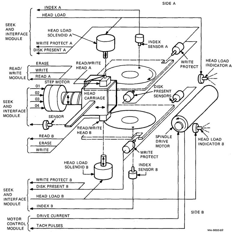
Figure 10-10 Mechanical Operation Detail
