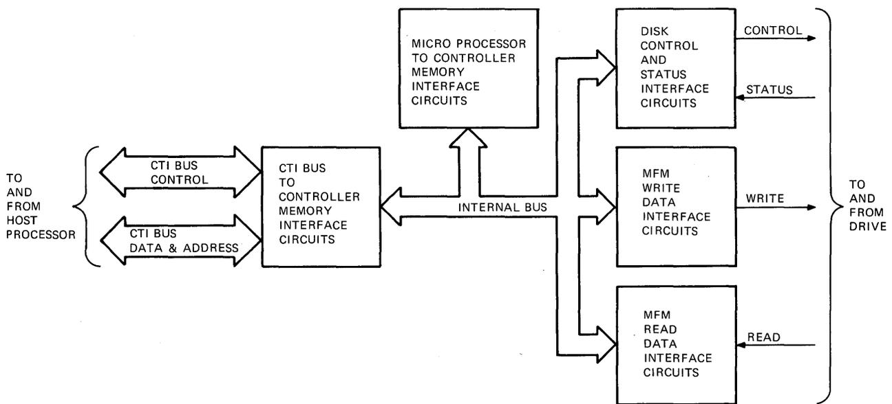
Figure 9-3 RX50 Controller Module Block Diagram
