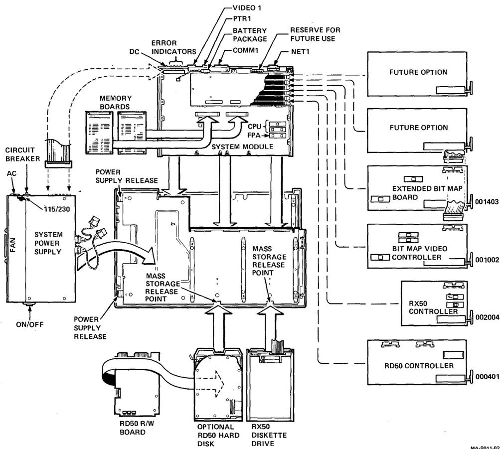
Figure 4-1 Physical Component Block Diagram
