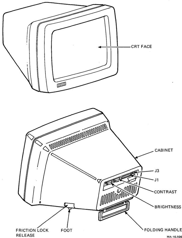
Figure 8-2 Monochrome Monitor Exterior View
