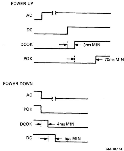
Figure 13-9 Power Status Signal Timing
