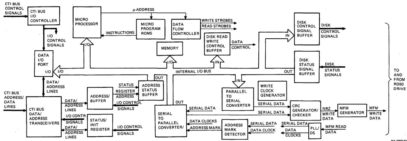
Figure 11-9 RD50 Controller Data Flow Diagram
