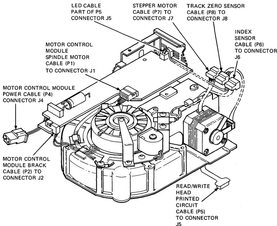
Figure 12-20 Internal Connection Locations
