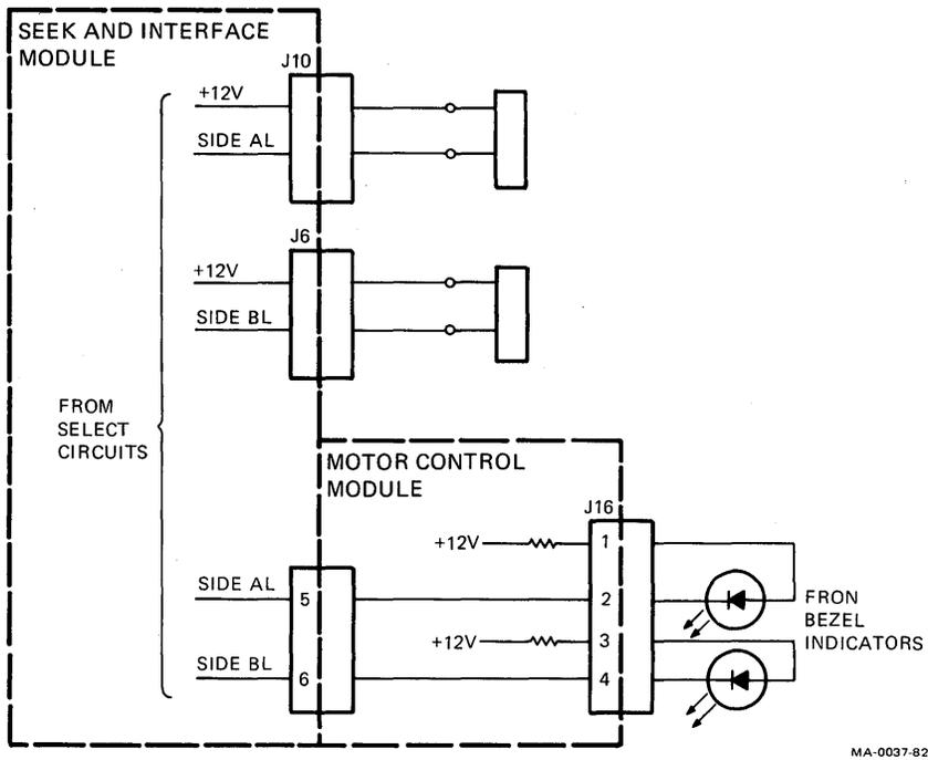
Figure 10-14 Connections to Head Load Solenoids and Indicators
