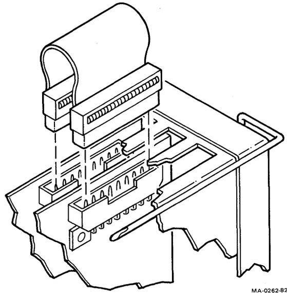
Figure 2-5 Bit Map Video Controller to Extended Bit Map Module Connector
