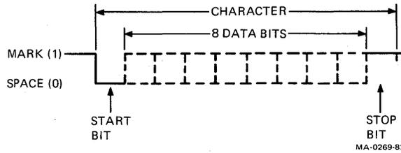
Figure 6-10 Keyboard Transmit and Receive Character Format
