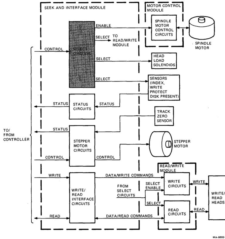
**10.3.2.1 Drive Select Circuit Detail** – The drive decodes the four drive select lines, DRIVE SEL 0 L through DRIVE SEL 3 L, depending on the condition of J17 (configuration jumper). With J17 open (without a jumper), the drive select circuit decodes DRIVE SEL 0 L and DRIVE SEL 1. With J17 closed (with a jumper), the drive select circuit decodes DRIVE SEL 2 L and DRIVE SEL 3.
