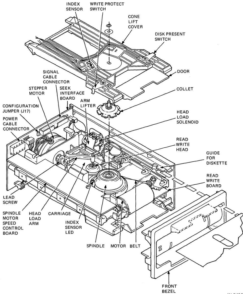
Figure 10-9 Mechanical Detail
