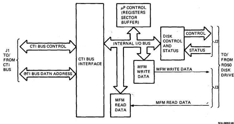
Figure 11-3 RD50 Controller Block Diagram
