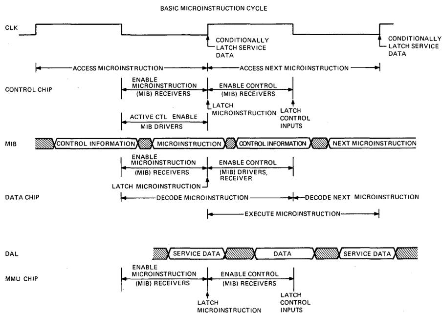
Figure 5-5 Basic Microinstruction Cycle
