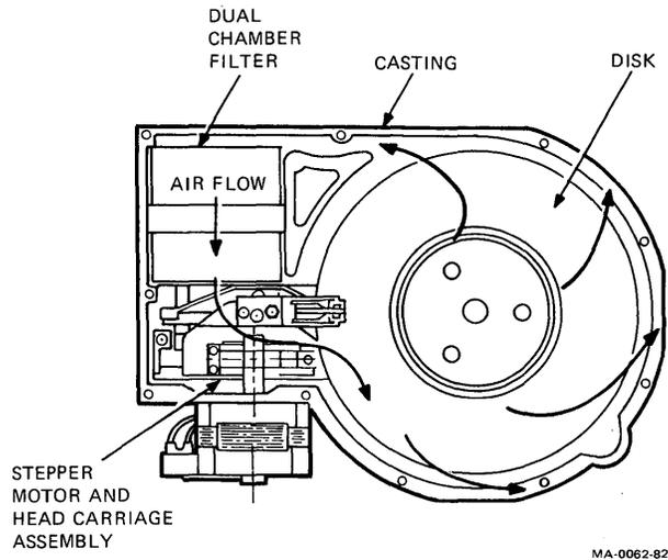
Figure 12-5 Air Flow Top View
