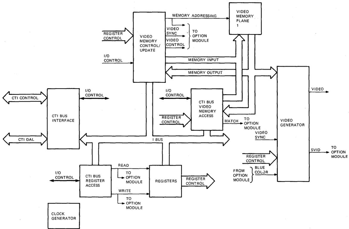
Figure 7-3 Bit Map Video Controller Block Diagram
