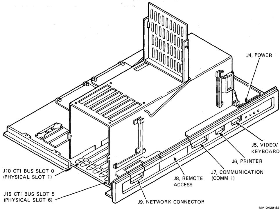
Figure 5-37 Connector Placement
