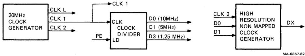
Figure 7-17 Clock Generator Circuit Operation
