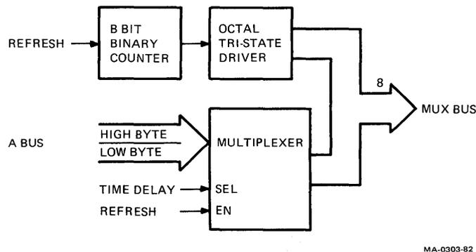
Figure 5-28 RAM Address Multiplexer
