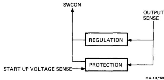
Figure 13-4 Control Block Diagram
