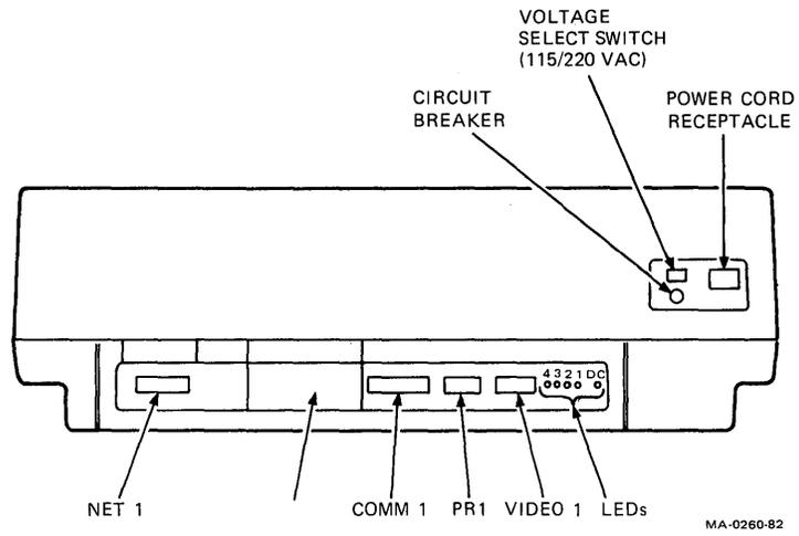
Figure 2-1 System Unit Rear Panel
