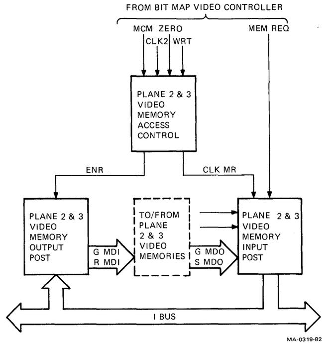
Figure 7-25 CTI BUS Video Memory (Plane 2 and 3) Access Circuits Operation (Option Module)
