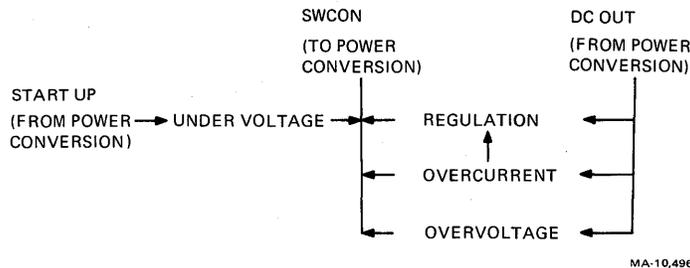
Figure 13-7 Protection Block Diagram
