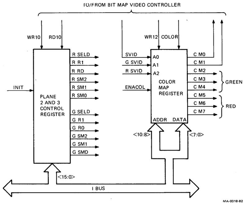
Figure 7-24 Plane 2 and 3 Control and Color Map Register Operation
