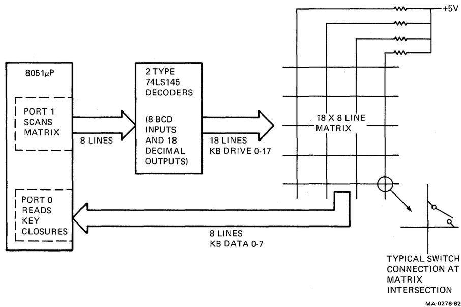
Figure 6-5 Simplified Block Diagram of Matrix Scanning Circuit
