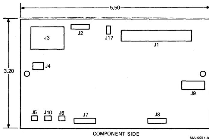
Figure 10-28 Seek and Interface Module Connector Locations
