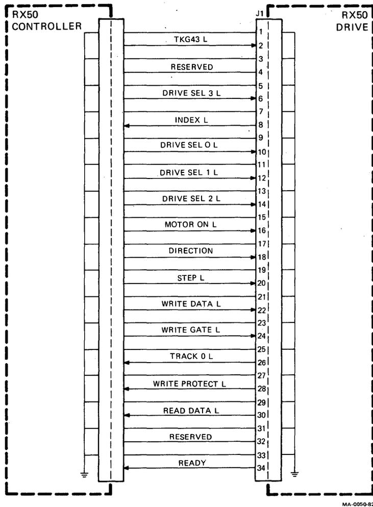
Figure 10-27 RX50 Controller and Drive Interface Signal Flow
