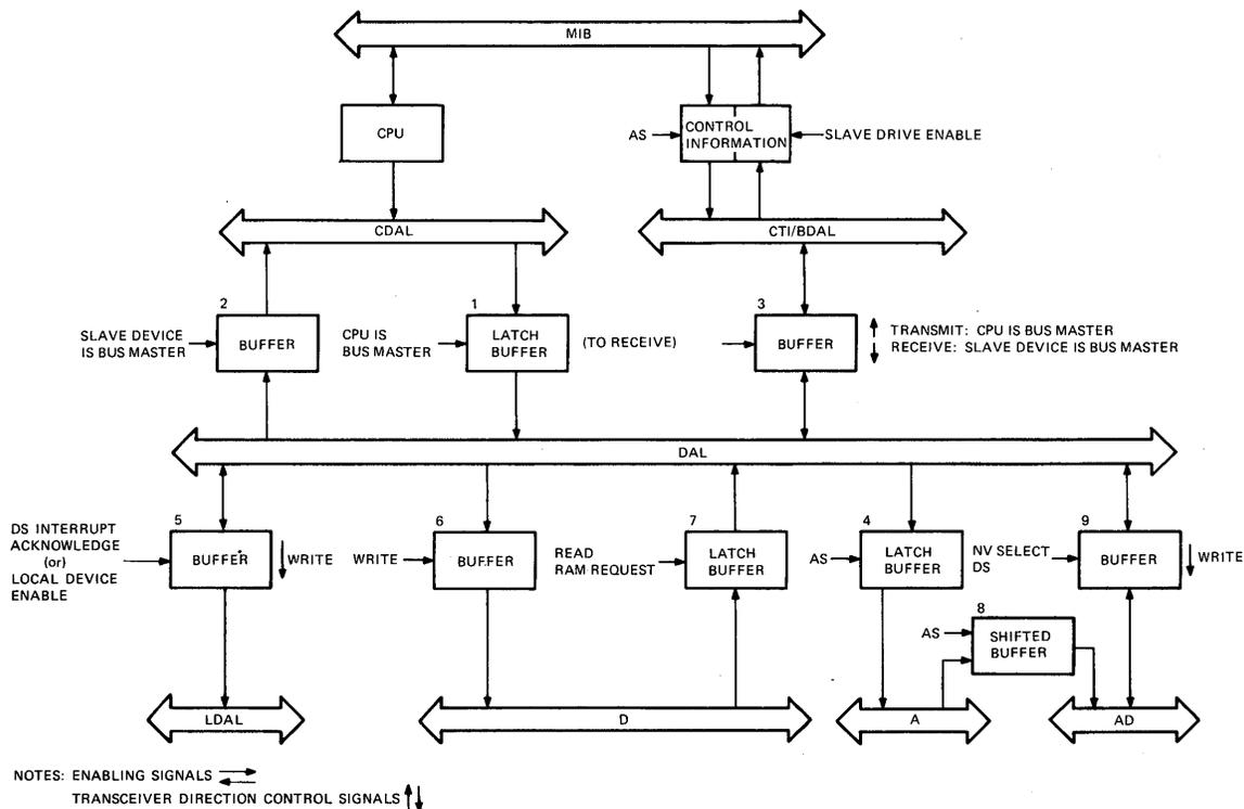
Figure 5-13 System Block Diagram with Bus Interfaces
