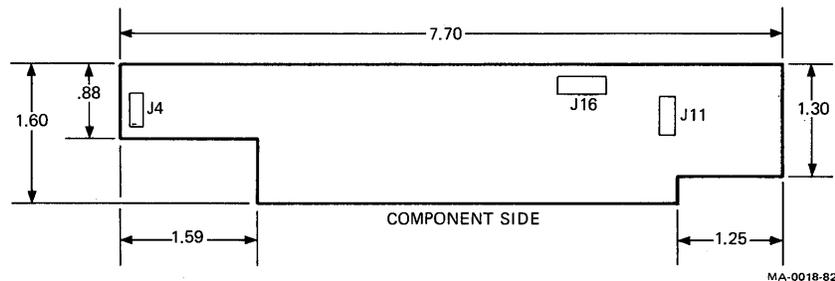
Figure 10-29 Motor Control Module Connector Locations
