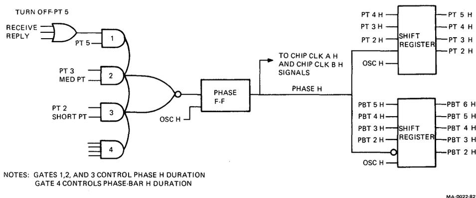
Figure 5-7 Phase Signal Duration Functional Diagram
