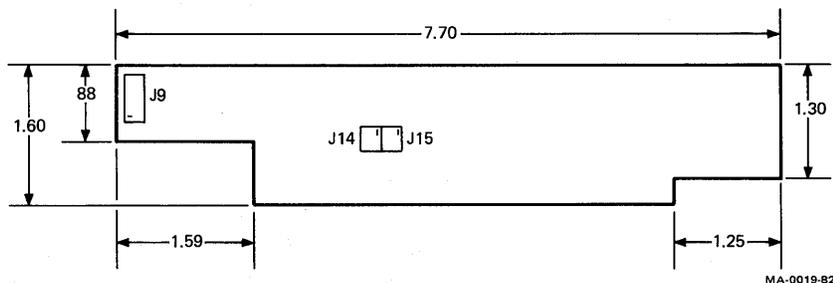
Figure 10-30 Read/Write Module Connector Locations
