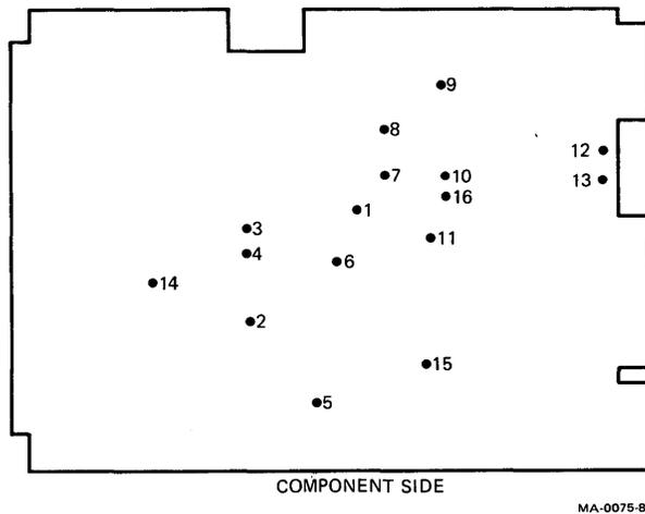
**Figure 12-21 R/W Module Test Point Locations**
