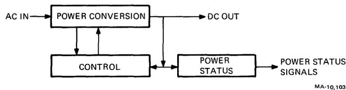
Figure 13-2 Power Supply Functional Block Diagram
