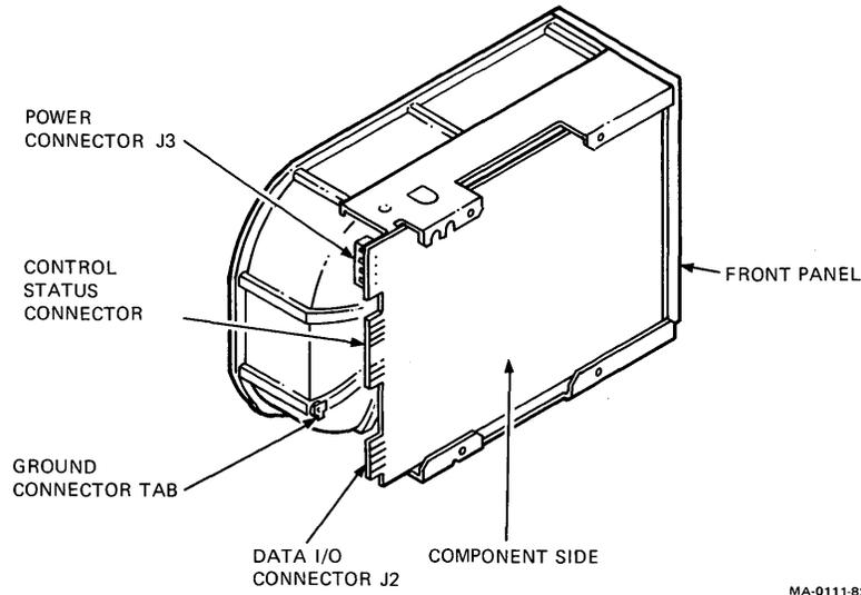
Figure 12-19 I/O Connector Locations
