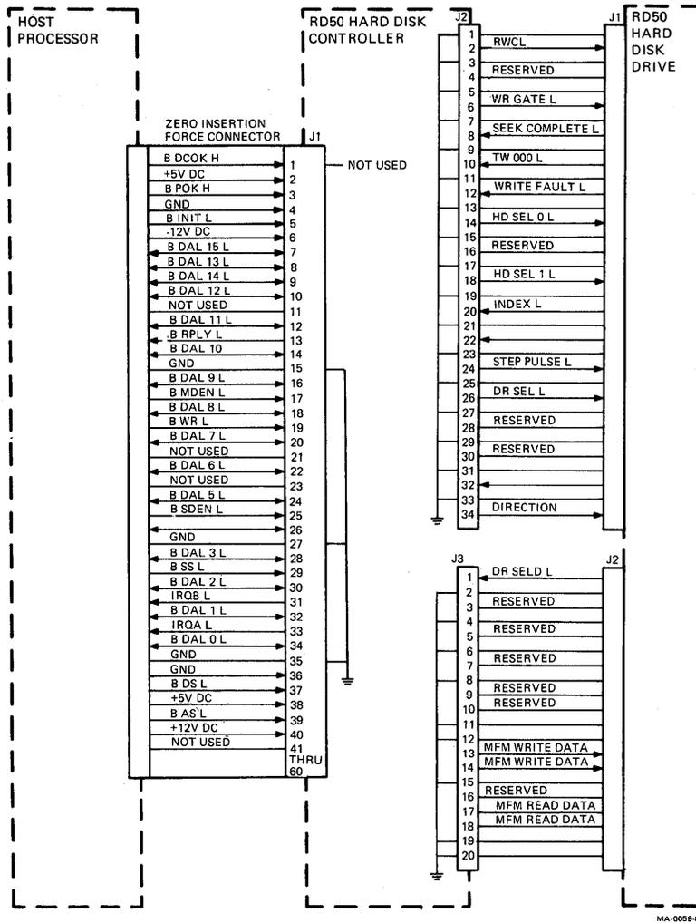
Figure 11-10 RD50 Controller Interface Signal Flow
