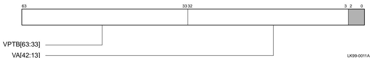
Figure 5–6 shows VA\_FORM when VA\_CTL(VA\_48) equals 1 and VA\_CTL(VA\_FORM\_32) equals 0.
