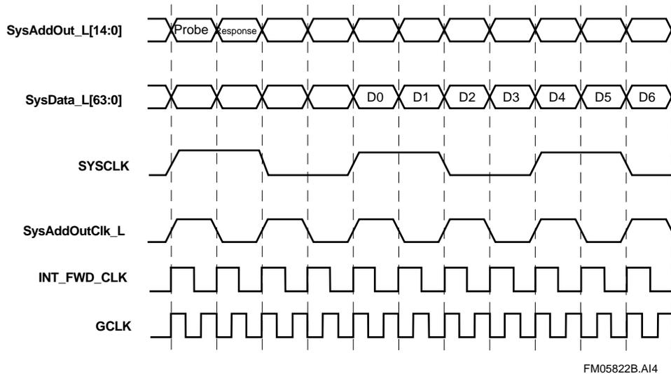
In fast data mode, movement of data into the 21264/EV68A requires turning around the SysData bus that is being actively driven by the 21264/EV68A. Given a SysDc fill command (ReadDataError, ReadData, ReadDataShared, ReadDataShared/Dirty, ReadDataDirty), the 21264/EV68A responds as follows:
