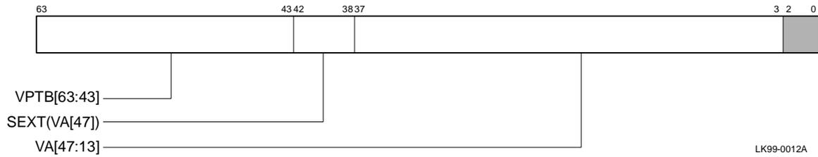
Figure 5–7 shows VA\_FORM when VA\_CTL(VA\_48) equals 0 and VA\_CTL(VA\_FORM\_32) equals 1.
