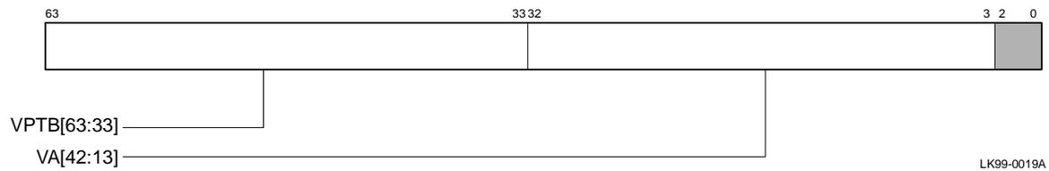
Figure 5–14 shows IVA\_FORM when I\_CTL(VA\_48) equals 1 and I\_CTL(VA\_FORM\_32) equals 0.
