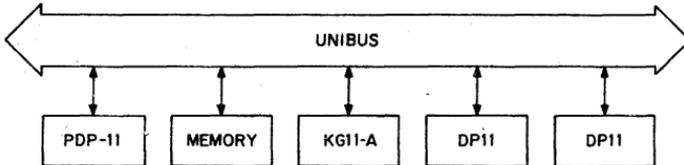
For received data, the characters are moved to the KG11-A and a BCC is computed for the data and compared to the BCC received. If they are equal, the data is assumed to be correct and is accepted. If they do not match, the message is not accepted and the data is retransmitted.
