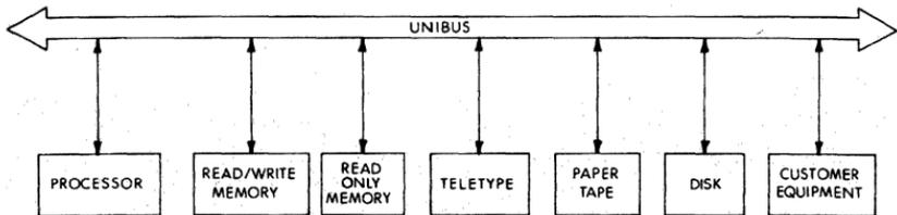
Figure 5.1 PDP-11 System Simplified Block Diagram
