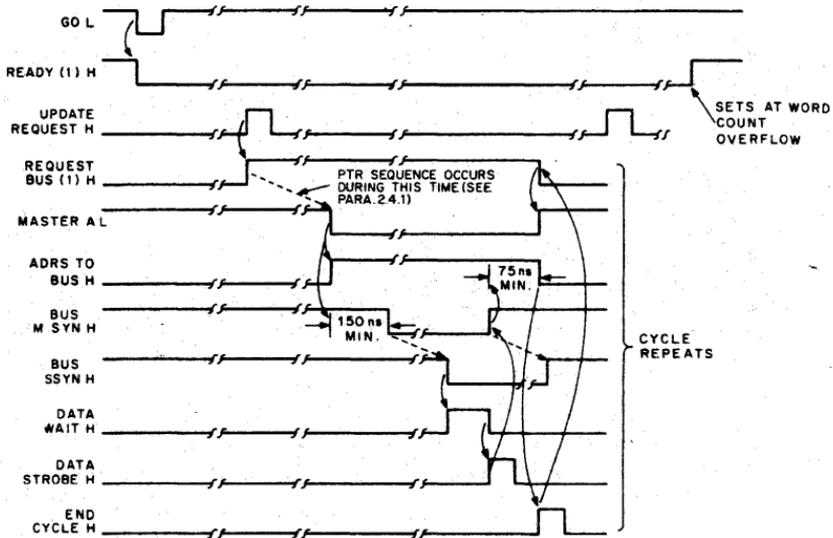
Figure 7-11 DAC-DMA Interface (timing diagram)
