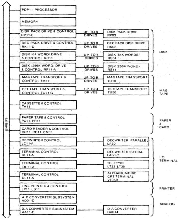
Figure 9-5 System Architecture of Major Components
