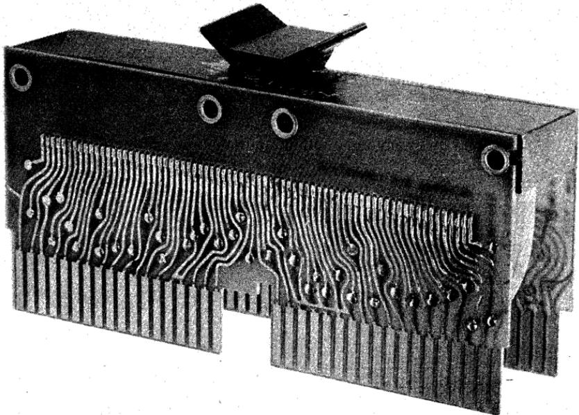
Figure 6-21 UNIBUS Jumper Module M920
