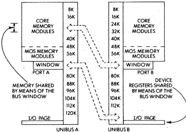
UNIBUS Window Operation Utilizing Both Window Ports
