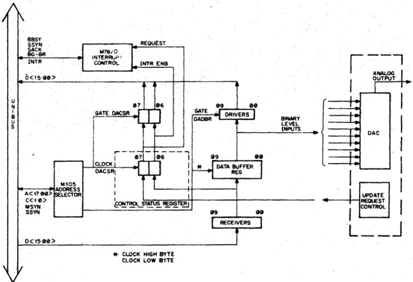
Figure 7-9 Output Interface with Interrupt Control (block diagram)
