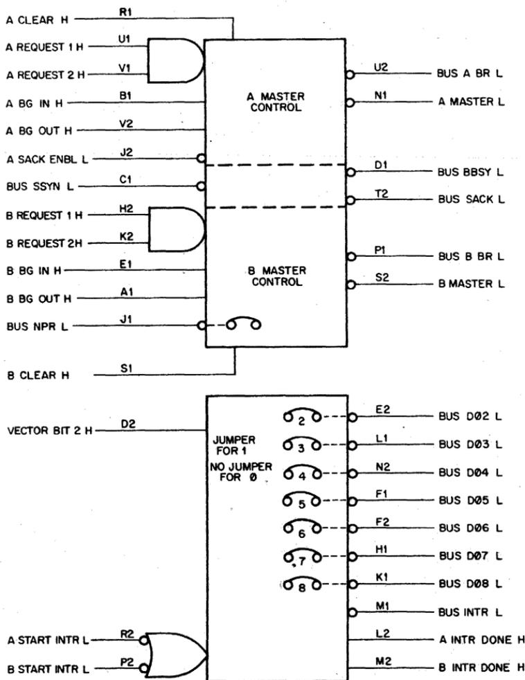
Figure 6-27 M7821 Interrupt Control Block Diagram
