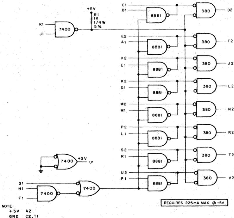
Figure 6-15 M785 UNIBUS Transceiver (schematic diagram)
