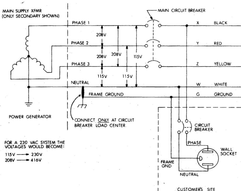
Figure 8-4 Power Wiring Schematic for 115 VAC
