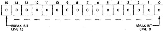
This register contains one bit for each line. Setting a bit in this register will immediately generate a Break condition on the line corresponding to that bit number. Clearing the bit will terminate the Break condition. The Break condition may be timed by sending characters during the Break interval, since these characters will never actually reach the line. Further comments concerning the transmission of Break signals may be found in the Break Signals Section.
