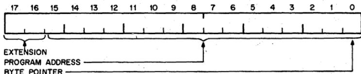
Figure 5-3 Address Line Bit Format
