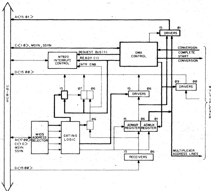
Figure 7-7 DMA Interface (block diagram)
