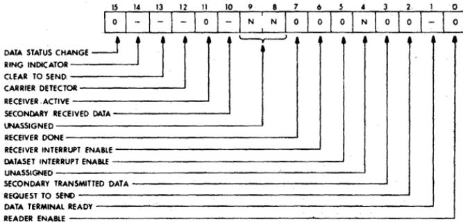
and by reading from RCSR. If bit 5 (Dataset Int. Enable) is set, the setting of bit 15 will cause an interrupt request to be generated.
