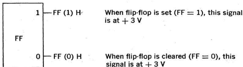
Figure 6-2 Flip-flop signals
