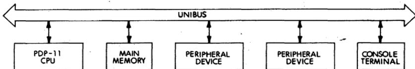
Figure 1-1 PDP-11 System Block Diagram
