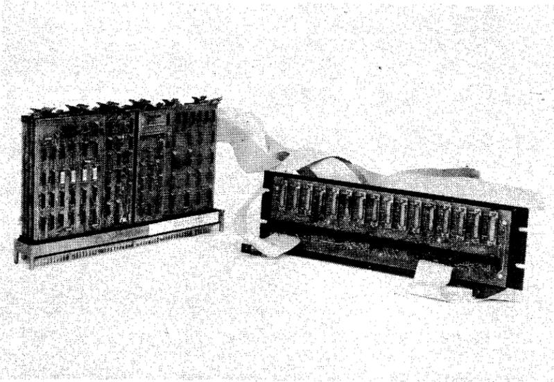
The DJ11-AB is supplied without level conversion, but with cables which bring the TTL signals out of the mounting cabinet. This allows connection to external signal-conditioning equipment, such as the DIGITAL-supplied DC08 Telegraph Line Interface Options, and customer-supplied special interface equipment.
