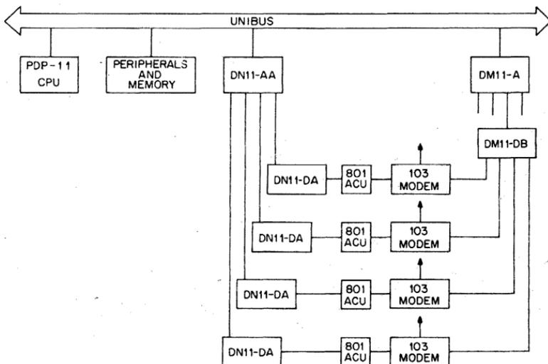
ASYNCHRONOUS MULTIPLE LINE INTERFACE
