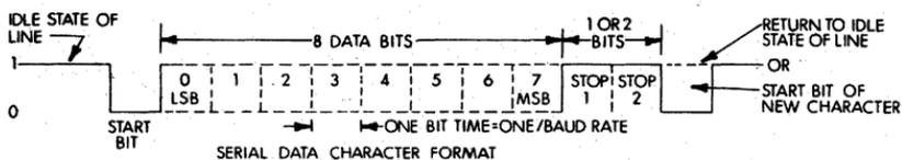
The 10-bit code consists of a start bit, 8 data bits, and only 1 stop bit. In addition to the LT33, the DL11-A can also be the control unit for a VT05 Alphanumeric Terminal, or an LA30-C serial DECwriter.
