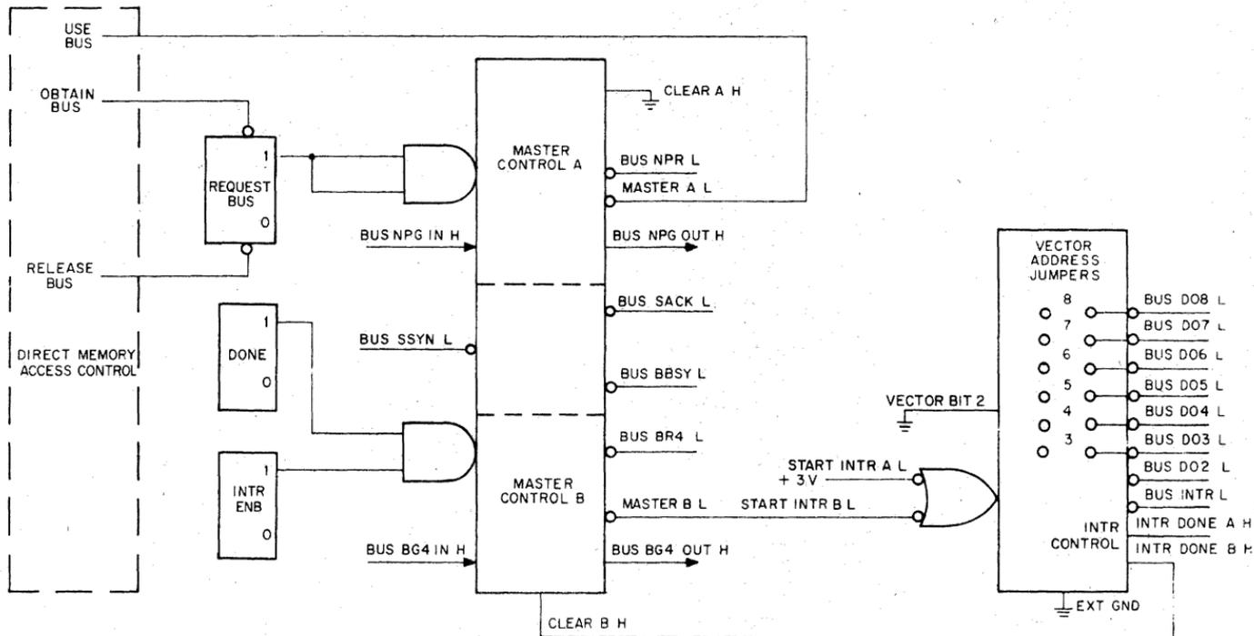
Figure 6-24 M7820 Interconnection for Direct Memory Access
