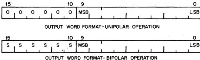
Bits 15 to 10 are tied together, and are "0" in the standard unipolar configuration. With the sign bit option, bits 15 to 10 indicate the sign of the input voltage.
