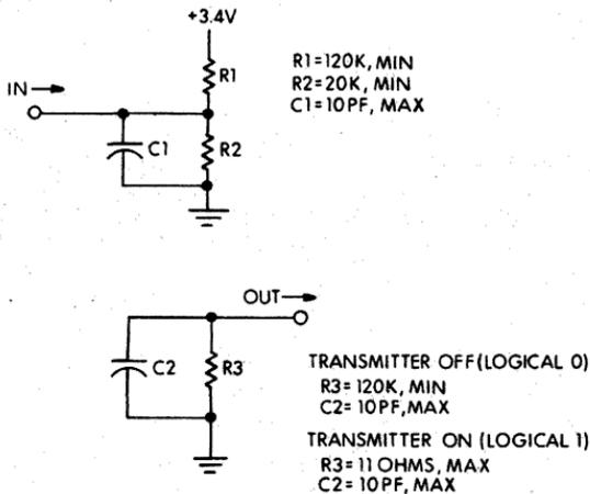
Figure 6-3 Transmitter and Receiver Equivalent Circuits
