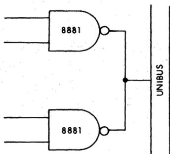
Figure 6-6 Wired OR Configuration
