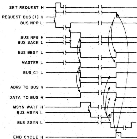
Figure 6-19 M796 Timing Diagram for DAT0
