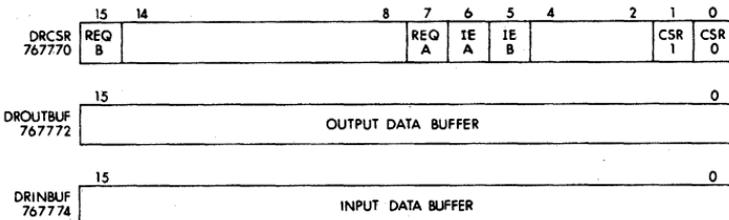
The register addresses can be changed by altering the jumpers on the address selection logic. However, any programs or other software re-
