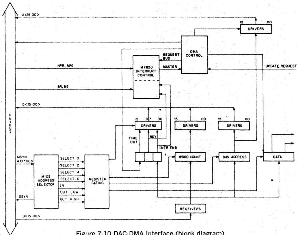
Figure 7-10 DAC-DMA Interface (block diagram)
