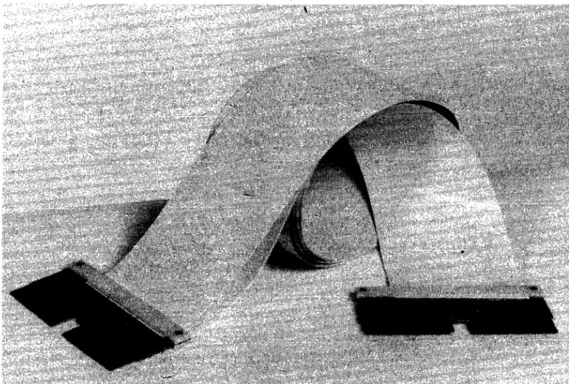
Figure 6-9 UNIBUS Cable BC11A
