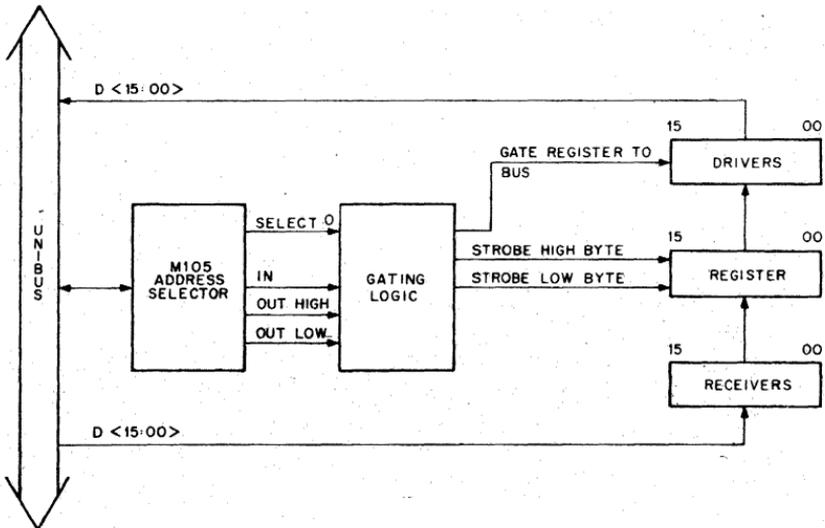
Figure 7-1 Basic Interface (block diagram)
