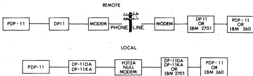
The DP11 can connect a wide variety of terminals to the PDP-11 either remotely or locally. These configurations would be:
