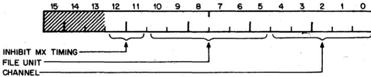
This Read/Write Register is for diagnostic purposes only. Permits checking of channel address by reading back decoded bits.
