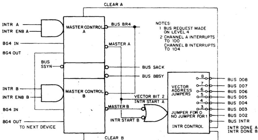
Figure 6-23 M7820 Interconnection for 2-Channel Interrupt
