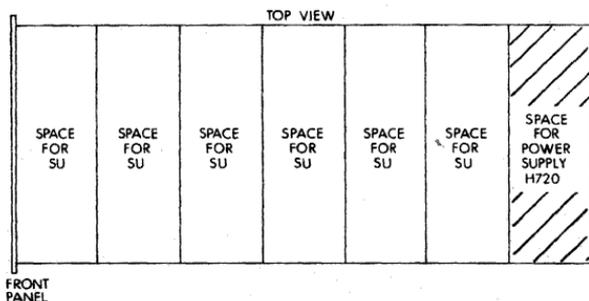
Figure 9-3 Extension Mounting Box (BA11)
