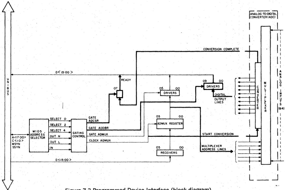
Figure 7-3 Programmed Device Interface (block diagram)
