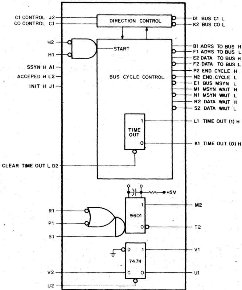
Figure 6-17 M796 UNIBUS Master Control (block diagram)
