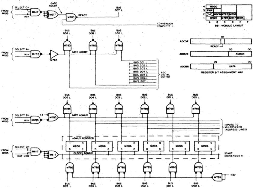
Figure 7-4 Programmed Device Interface (schematic diagram)
