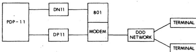
The DP11 also can connect two PDP-11's together or a PDP-11 to another large processor (e.g., IBM 360). These connections which could be either remote or local would appear as:
